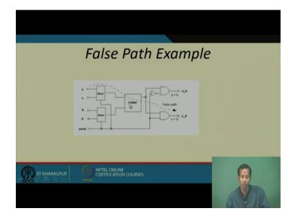
So, then this, what is the false path example is that? Suppose as we are having a b c d and we are having this condition. So, depending on this condition as there are; that means, all the paths are basically connected from a to b or c to this d d b to this d to this, but this particular path will be never activated. Depending on the logic this particular path will be never activated which will follow that a to this. So, that is why this path is named as or this path is called as false path.
