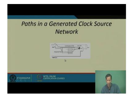
So, then the paths which are there in the generated clock source network is that you will be having one combinational path, you will be having one sequential path and in this clock signals will be just connected to this sequential elements passing through some inverters or some buffers.
