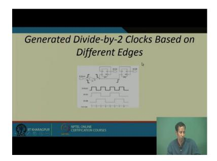
So, now, how you can generate divide by 2 clocks based on two different edges. So, suppose you are having this system clocks, now you just pass this system clocks through one inverter where this will be just; that means, negative unate clock. So, now you just this negative unate clock directly you just pass it to this one of this flip flop and another with inverted clock.
