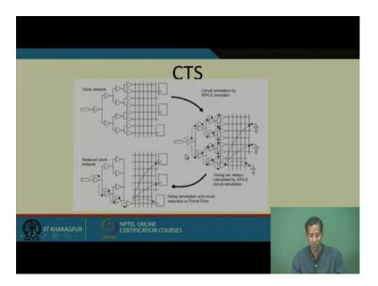
So, this is this clock tree synthesis so; that means, this is the clock source pin then it is connected as H tree ok. So, you see from one buffer then again it is connected with two buffers then again two then again it is distributed two and again by this will create the
