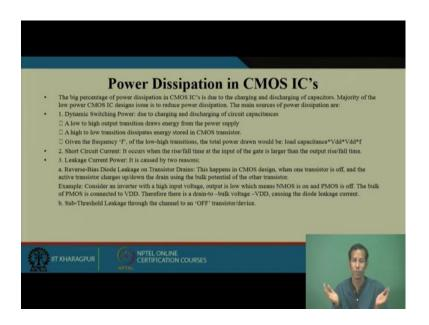
So, in actually CMOS IC design we are having different kind of source of power dissipation. So, you will be having this dynamic switching power consumption, you will be having this short circuit current power consumption, you will be having this leakage current power consumption so, all these are there.
