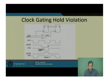
So, then again actually we are we can get some of the; that means, this is some of the configuration where we can get because of the hold time we can get the glitch at the clock 2 and that can create a problem in your circuit.
