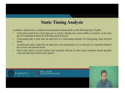
So, why to consider is that, there may be this kind of paths more than one path will be available from input to the output. And, every of this timing information of every of this path you have to calculate using static timing analysis. Unless and until if you miss any one of this particular path and it creates or it associate with the corresponding violation. So, at that time your chip will not work it may fail to perform successfully ok.
