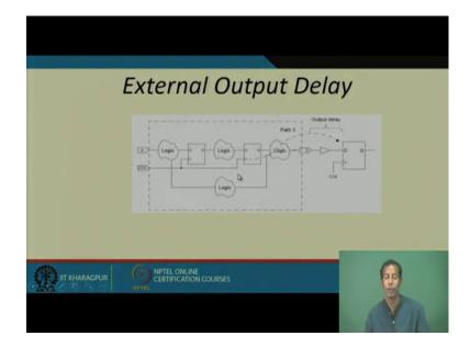
Then again you have to set the external output delay. So, the external output delay will be the clock pin of your final registers to the clock pin of the; that means, the output side at the output side, what flip flop you have used that means the first flip flop to its where it is connected ok.
