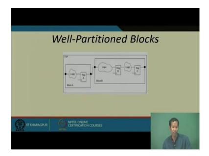
So, at that time what I do is that, I put the corresponding block A; that means, all this logic I just place to block B ok. And, I am having only logic and registers A over here and I am having the logic and then all this part over here.
