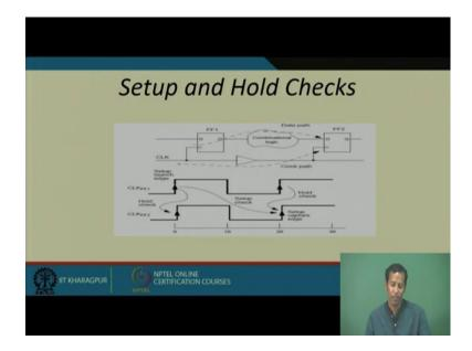
So, this is the setup and hold check at this particular edge, you have to consider thus; that means, hold check as well as; that means, for the setup check for both flip flop 1 and flip flop 2.
