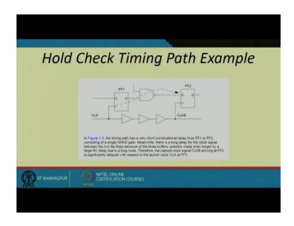
So, again we will see that how; that means, in the previous lecture we have seen the set up how we perform the set up timing check in the corresponding circuit. So, now, we will see the hold time check for any particular circuit.
