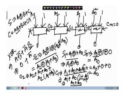
So, for that what we have done in the incrementer design. So, do the same thing we have to do in this case also. So, that means, here if I consider; that means, each of this as that means, 4 bit means 4 full adder cell I require. So, this is A 3 this is A 2 this is A 1 this is A 0 and this is the carry which is been forwarded to the MSB side and this carry is basically cancelled, that means, I am discarding this carry out.
