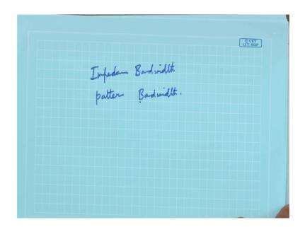
That means antennas impedance should be at least within let us say that how much more sometimes you know KSWR is a measure of impedance with respect to a standard particularly with a characteristic impedance of the transmission line. So, impedance bandwidth is a term. That is why we will see that many antennas people characterize ok; the 10dB impedance bandwidth; that means, our VSWR is or reflection coefficient 10dB. So, actually that is a characterization of impedance bandwidth.
