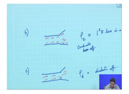
The second part will be that in the antenna; in antenna there are some metallic structures some conductors, so obviously, if electrons flow from there as a current then there will be some resistance, so that will there will be some loss.
