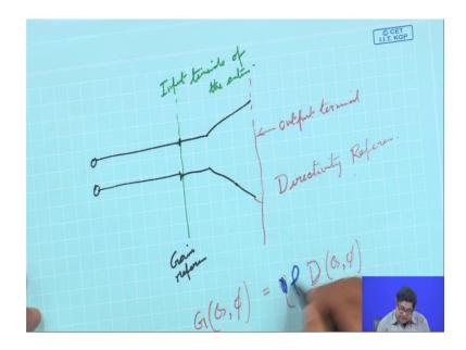
That is suppose I have a radiating antenna. So, we can say that this plane here we can call this as the something like output terminal of an antenna, because after this the web is being launched in free space. So, this is basically the directivities reference. That means, in the denominator of directivity function basically we say that power radiated by an isotropic radiator; that means, this radiation is taking place here. So, this plane is the directivities reference.
