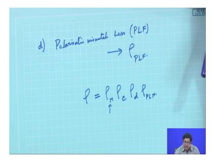
If polarisation is match then there will be maximum power can be extracted. So, polarization mismatch loss this is PLF. So, this gives rise to an efficiency which is called rho PLF. So finally, we can say that that rho is nothing but rho r rho c rho d rho PLF.
