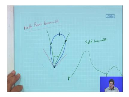
Now you see this also, because generally we have seen when the radiation pattern of an antenna that the there is a main beam generally associated with each antenna. So, most of the power is concentrated into the main beam. So, that is why how wide is that beam that is an useful criteria. So, if I have a very short beam, but I have sufficient power then that is good; that means, the antenna is very reactive. So, that is why people have come out with this that.
