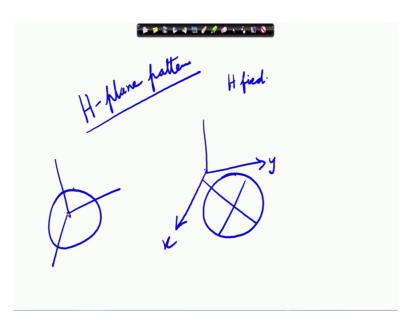
H-plane pattern means the direction of maximum radiation, again that y axis and the H field. So, what is the H field? That is the Azimuthal field and this direction of maximum radiation y so, the field is like this. So, in the x y direction if we plot we have seen that that will be a circle; sorry I will have to center it like this circle. So, everywhere this is same that we have already seen this way this is not correct, this will have to be centered. So, that is called H-plane pattern.
