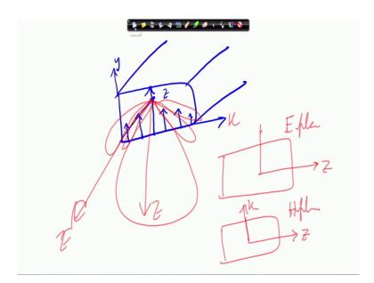
Similarly, if instead of this suppose I have a rectangular waveguide at the radiator many times this happens. In the rectangular wave guide in the dominant t 1 mode you know that electric field is like this, this goes to 0. So, electric field is in this direction; let us say that this is our y direction this is our x direction and this is our z direction that one. Now, so it is easy that maximum radiation is taking place in case of open handed wave guide the maximum sorry.
