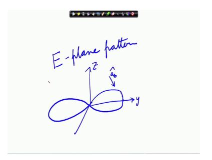
So, if we plot that that is called E-plane pattern. So, we are plotting that radiated power in the plane called E-plane. What is the E-plane? E-plane is the plane made by the electric field and the direction of maximum radiation. In case of current element, if you recall in case of current element the direction so, if we are here this is our z axis. So, the direction of maximum radiation was y axis in this direction and electric field that is in the theta direction.
