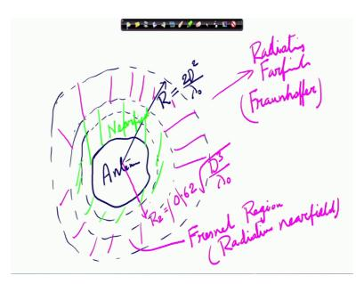
So, actually the region suppose this is the region of the antenna, suppose this is antenna. So, we can draw that from this a at a distance of we can call R, this R is 2 D square by lambda naught roughly, this is an nowadays acceptable criteria that far field starts. But what happens in between? In between also there is another region, another actually two regions. So, I will draw like this let me choose another colour. So, there is another distance let me call this there are two regions.
