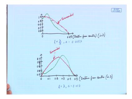
But people have found out experimentally also. And also by other techniques that it is not exactly sinusoidal. Look at the top graph it is for a lambda by 2 dipoles. It is a thin dipole, because the usually dipoles radius is quite small in terms of lambda. And here in the x-axis is plotted the distance from the center, so that means this is the central point, and this is the top point. And the current distribution is symmetric in both the poles.
