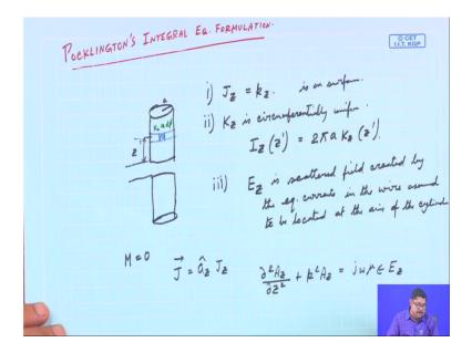
So, we will see now that that Pocklington's integral equation formulation, again we have that cylinders. Here the current density is on the surface. So, the first assumption of this is the current density J j is on surface. So, it is called k z that, now the second thing is this surface current density k z is circumferentially uniform.
