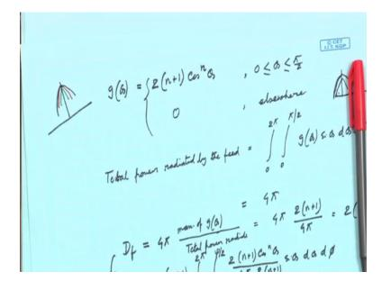
Suppose, the feed radiation pattern is something like 2 n plus 1 cos n theta; that means, instead of sec 4 theta we take cos theta some power for 0 to theta to phi by 2, so, in this zone and 0 elsewhere. Now, this factor 2 n plus 1 that is chosen for a reason that we can see that if a feed has this power pattern, what is the total power radiated? So, the total power radiated by the feed that will be 0 to 2 pi 0 to pi by 2 then d theta sin theta d theta d phi.
