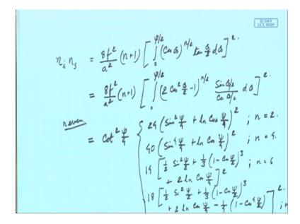
So, we can write that from here I can write eta i eta s is 8 f square by a square n plus 1 0 to psi by 2 cos theta n by 2 tan theta by 2 d theta whole square. So, this needs to be maximised. So, this people have further make it. Now, this integral is 0 for odd n and non zero for even m. So, this can be written as cot square pi by 4; then its value people have evaluated that. So, only for n even this is non zero.
