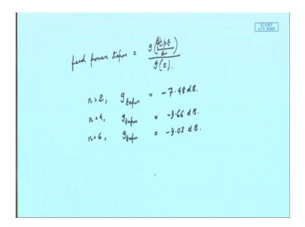
So, feed power taper because the designer of the feed is this value that will be given by g sorry psi opt by 2 by g 0 and. So, this for n is equal to 2 we can write g taper will be. So, this value was 130 degree. So, g of 65 you can put it and please remember here it will be 10 log d because it is a power pattern. So, these becomes minus 7.48 dB, n is equal to 4, g taper becomes minus 9.66 dB, n is equal to 6, g taper becomes minus 9.03 dB ok. So, that shows you the thing.
