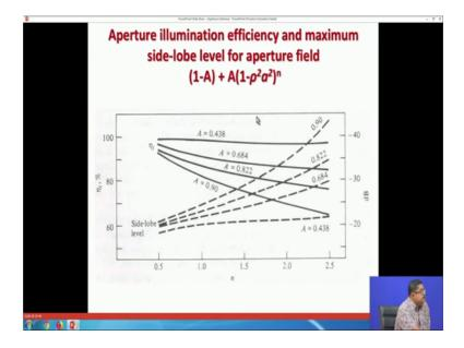
Aperture illumination efficiency; that means, eta x and maximum side lobe level for aperture field, so, for a eta i how much you get? So, you see that if we take the this aperture taper to be more and more for then you see that illumination efficiency that
