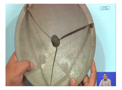
Here, you can see this is actually a paraboloid dish, this is the horn feed; you can see the horn feed here. This is the horn this is the circular horn instead of a rectangular horn, it is at the focus and aperture means this circular zone. We see this is the circle here; hypothetical circle that is the aperture; that is diameter is being said. So, f by d ratio
