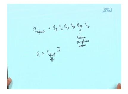
So, that will be one is spillover efficiency, one is illumination efficiency, one is polarisation efficiency, one is uniform field efficiency, then this surface roughness, this is surface error; surface I will say roughness error efficiency and then the blocking efficiency. So, all this effects the aperture efficiency. So, finally, gain is nothing but eta aperture efficiency into the directivity of the aperture ok.
