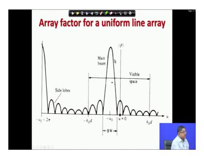
You see that it was in between, the main beam was in between. Here, it has gone through one extreme. So, there is high chance that the next one can put to for a array end-fire array. So, we will have to find out that to avoid grating lobes what we can do? We know that the array factor is a periodic function that we have said that array factor is periodic with a period 2 pi.
