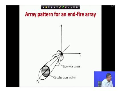
And so, we can see how the thing looks like; array pattern for an end-fire array is looks like this. These are the side lobes. So, you see x axis is the array axis and the main beam is along the array ok. It is a figure of revolution about the array axis and we now need to find out the other parameters of this, the array factor we can write. What is the array factor of end-fire array? That is I naught sin n plus 1 by 2 k naught d. You see that u naught I will put this thing.
