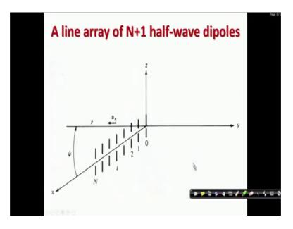
So, this you see that I can say here again, you can see the that this is dipole but it could have been anything, here without loss of generality we are assumed dipoles this could have been monopoles this could have been horn antennas this could have been opponent guide antenna etcetera etcetera. Now to see that the elements are placed along x axis a line and there are N plus 1 such elements because, first one we are naming zero 12
