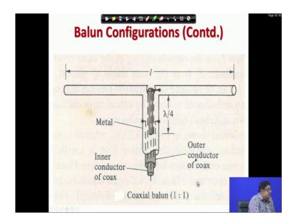
And this is this third configuration. So, this one is outer conductor this the inner conductor coax inner conductor this one I think this is now. So, Balun then what it actually is job is now to make this balanced to unbalanced this unbalanced comes.
