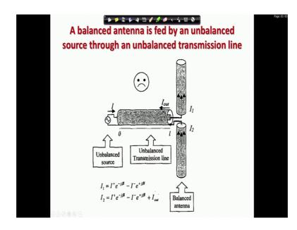
Now, how do we connect them to the thing? You see; obviously, you see this is a to prevent the radiation from the transmission line. What we do? There is an outer shield and that outer shield is connected to the lower half and the inner conductor that is taken out the direct conductor is put here.
