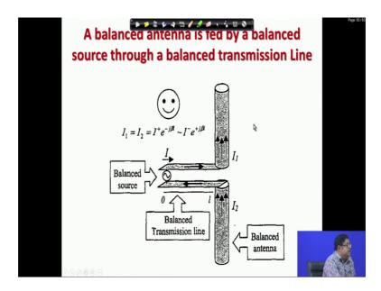
The next one is, but this is not practical the earlier case that was not practical because I cannot put the source into the center of the antenna; basically source is at a distance. So, to do that there is a transmission medium or transmission line and if we have two wires, so, I have a source again a balance source, I have a two wires and one of the wire is connected to the upper hub the another wire is here.
