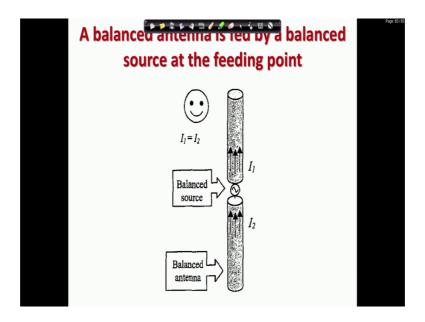
If these two poles assume same current distribution the radiation efficiency is maximum, the current should go in one direction and the same current should return to the other one. The goal is to feed the antenna in such a way that these two poles have exactly the same current distribution that is the even symmetric.
