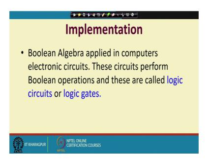
So, that gives that gives the impetus like why the why should we work on this, on Boolean algebra for this logic circuits. So, Boolean algebra is applied in computers and electronic circuits and these circuits perform Boolean operations using something called logic circuits or logic gates. So, we will see the some elements. So, logic gates are again you can say it is some sort of electronic structure. So, that can that can implement in AND operation, OR operation, NOT operation like that.
