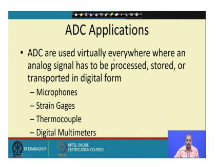
So, ADCs are used virtually everywhere, where an analog signal has to be processed stored or transported in digital form like microphones, strain gages, thermocouple digital multimeters. So, everywhere you will find some application of ADC; so, ADC.
