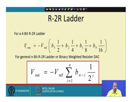
So, we have got this V out is this is the final expression that we have. So, V ref into b 3 into 1 by 2 so, this taking that R f equal to R by 2. So, we get it V ref equal to b 3 into 1 by 2 plus b 2 into 1 by 4 b 1 into 1 by 8 plus b 0 into 1 by 16.
