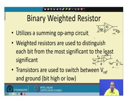
The first binary so, first digital to analog converter that we look into is the binary weighted resistor based digital to analog converter. So, you utilizes a summing operational amplifier circuitry. So, what we mean by a summing operational amplifier is so, operational amplifier is some circuit like this I hope your familiar with the this diagram.
