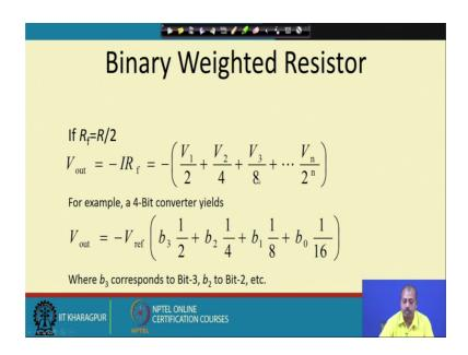
Now, if we so, if R f equal to say R by 2. So, if you take R f equal to R by 2, then this V out equal to minus I into R f which is V 1 by 2 plus V 2 by 2 plus V 3 by 8 up to V n by 2 to the power n. So, then we can say that this if you have got say 4 bit converter, then this V 1 is nothing, but V ref this V 1 V 2 V 3 they are all equal to V ref. So, this V ref is taken out.
