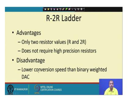
So, why should we go for R 2 R ladder? So, advantage is the only 2 resistor values are necessary which is R and 2 R and does not require high precision resistors.
