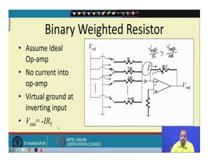
So, this is the structure you can say. So, each of this bits that we have so, each of this lines so, they constitute 1 bit fine. So, you can see that we have we have got we have got this operational amplifier like this bit. So, if it is a so, this bit. So, if I connect it to this point. So, this V ref the current that is drawn by drawn by this is V ref divided by R.
