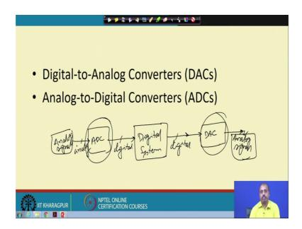
So, in this part of the course so, we will be looking into 2 such converter mechanism one is called digital to analog converter or DAC, and another is known as analog to digital converter or ADC.
