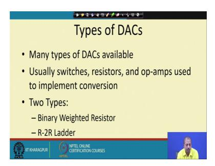
Now, if you look into these types of these digital to analog converters. So, there are many types of DACs that are available. And, they are usually switches resistances and operational amplifiers; they are used to do this conversion. And, there are we will be looking into 2 type of DAC one is known as binary weighted resistor and R 2 R ladder type resistor.
