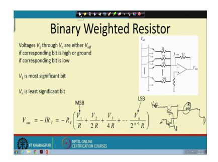
So, this is if the connection is like this. So, this point is connected to V ref this is connected to ground and we have got a switch. So, this is connected to the digital bit V.
