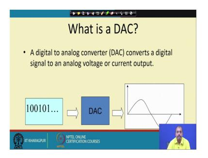
So, what is DAC? A digital to analog converter it converts a digital signal to an analog voltage or current output. So, because voltage and current they are they do not cause much of problem, because if we get a current output also so, we can pass it through a resistance and then measure it the corresponding voltage. So, as a result is current and voltage. So, these 2 outputs any of these outputs are with us.
