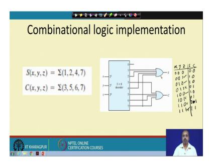
Now, this decoders they can be used for realizing combinational functions directly for example, suppose we look into that adder function ok. So, in case of adder you know that the sum is given by sigma 1 2 4 7. So, this x y z it is a full adder.
