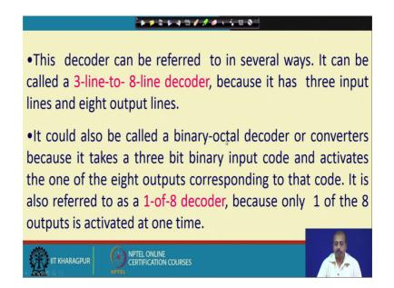
This decoder can be referred to in several ways; first of all it can be called a 3 line to 8 line decoder. As there are 3 input lines and 8 output lines. So, it has it is called 3 line to 8 line decoder. Now see this 3 and 8 so, these information they are redundant like as soon as I say the 3 are the input lines. So, 8 are the output lines.
