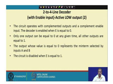
So, next we will look into so, this the circuit operates with complemented outputs and, a complement enable input as we have said. So, the output active output is 0 and, decoder gets enabled when E is equal to 0. Only one of the can be equal to 0 at any given time all other outputs are equal to 1, output whose value is equal to 0 represent some min term selected by inputs A and B.
