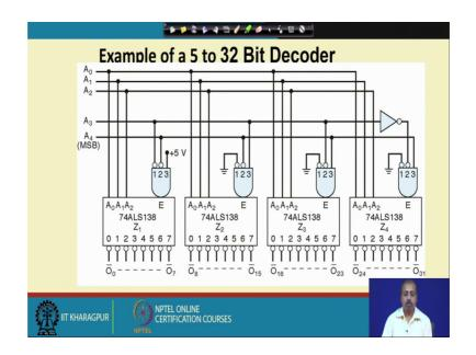
Next we will look into how can I make a five to 32 bit decoder using this 3 to 8 decoders ok. So, so, I want to make a hierarchical structure so, in my application I need a 5 to 32 decoder whereas, in my library I do not have this 5 to 32 decoders available as a chip, what I have are only 3 to 8 decoders 7 4 1 3 8.
