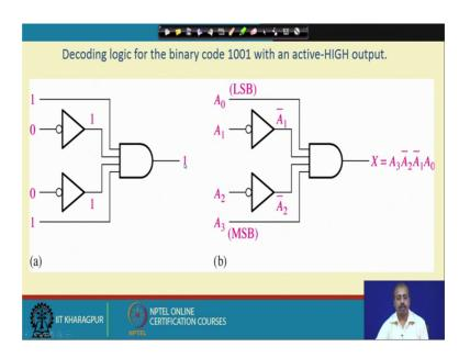
So, here I was look for active high output, so, I could do that using inverters and AND gate. So, if I was looking for active low output, then I have to use inverters and NAND gates.
