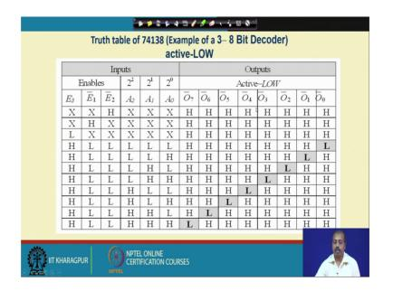
So, this is the truth table for 7 4 1 3 8. So, this is when this E 3 is so, when whenever this is a E 2 is high. So, E 2 bar becomes low so, this your decoder is disable. So, all the outputs are high, or if E 1 is high whatever be the value of E 3 and E 2, then also all the outputs are high. And if E 3 is low whatever be the value of E 1 and E 2 so, again all the values are all the all the outputs are high.
