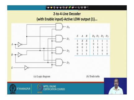
So, the first one we will be considering is a 2 to 4 line decoder with enable input. So, what is there so, so here, this is the 2 input A and B that are the, that gives us to the output number that should be made active ok.
