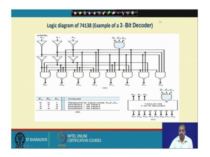
So, next we will look into the logic diagram of this integrated circuit chip 7 4 1 3 8. So, this 7 4 1 3 8 is a 3 bit decoder. So, we have got A 0 A 1 A 2 as the input and, it is when this so, it has got a number of enable line. So, this E 1 E 2 and E 3, there are 3 enable lines out of that the circuit is active when E 1 bar is E 1 equal to 0 that is E 1 bar equal to 1 E 2 equal to 0 that is E 2 bar equal to 1 and E 3 equal to 1.
