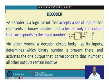
So, a decoder it is a logic circuits that accepts a set of inputs that represents a binary number and, activates only one of the output that corresponds to the input number. So,
