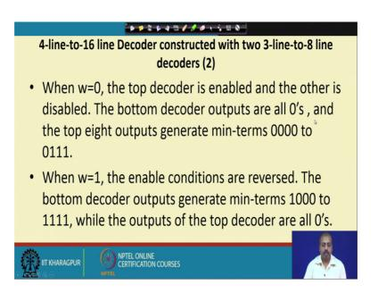
Next we will be looking into how can I get 4. So, this is the description of that 4 to 16 line decoder. So, when w equal to 0 top decoder is enabled and the other is disabled and, the bottom decoder outputs are all 0's because, the EB the enable input is 0 and, the top a and top 8 outputs generate min terms  $0\ 0\ 0\ 0\ to\ 0\ 1\ 1\ 1$ .
