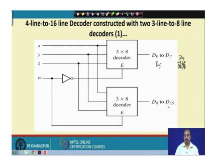
A simpler example how to construct a 4 line to 16 line decoder using 2 3 line to 8 line decoders so, we have got two 3 to 8 decoders and we use them to get a 4 to 16 line decoder. So, we assume that each of this decoders they have got one enable line and, for the decoder to operate this enable line should be equal to 1 ok.
