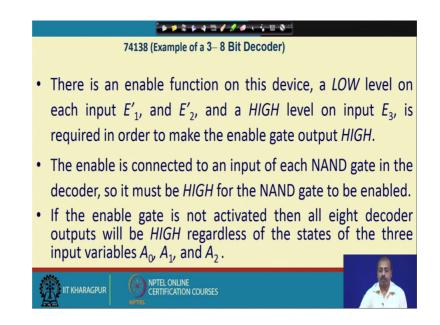
So, there is an enable function on this device a low level on each of the E 1 dash, E 2 dash, and E 2 dash and a high level on input E 3 is required to make the enable gate output high and the enable is connected to an input of each NAND gate in the decoder. So, it must be high for the NAND gate to be enabled, if the enable gate is not activated, then all the 8 decoder outputs will be high, regard less of the states of the 3 input variables A 0, A 1, A 2. So, that is for the enable part.
