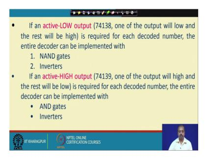
As I said that there can be two variants of the decoder one decoder is active low output, where the whichever output is active. So, that output will be 0 and the rest will be 1. And other category is active high output, where I have got this decoder who the active output will be 1 and the rest will be 0.
