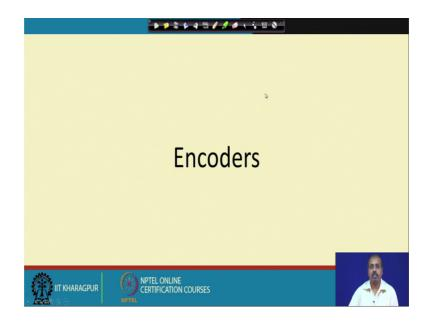
So, next we will be looking into encoders. So, encoders just the reverse of decoders so, in case of encoder decoder from less number of line so, you are going to more number of lines, for the encode will do just the reverse, we will start with the more number of lines and from there we will come to less number of lines.
