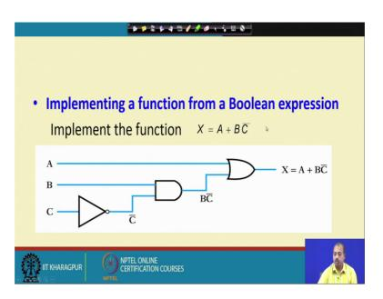
So, suppose we have got Boolean expression X equal to A plus B C bar ok. So, to how can we realize in terms of logic gates. So, you see that this OR so, fine at the highest level we have got this OR operation ok. So, we so, at that at the output at the top most level. So, we will have this OR gate so, OR gate will have 2 inputs. So, this A input and this B C bar inputs. So, input is connected to first input of OR gates and this B C bar will have to the second input of OR gate.
