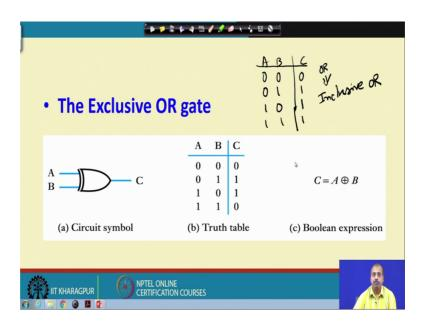
So, next we will look into the another derived gate which is known as exclusive OR gate. So, if you remember the OR gates. So, it was like this so, the truth table for OR gate was the A B and C, whenever the whenever any of the inputs was equal to 1. So, this was equal to 1 so, 1 0 is the also 1 and 1 1 was also equal to 1. So, this was the truth table for OR gate.
