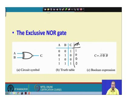
So, next we will look into the inverted version of X OR which is known as X NOR gate exclusive NOR gate. So, this is NOR but exclusive. So, NOR gate was that whenever we have got any of the inputs equal to 1 output was equal to 0. This is the difference in X NOR gate when both the inputs are equal to 1. So, output is equal to 1 so, this is not equal to 0.
