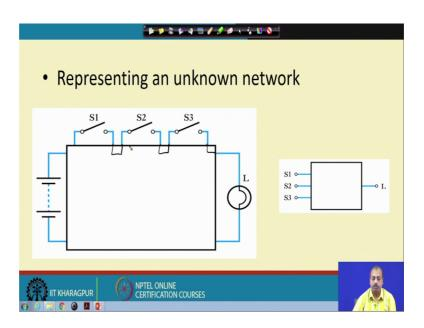
So, now, if we suppose we have got an unknown network ok. So, this is a black box so, this is a black box I do not know what type of connection we have between these points. So, this say from this output of S 1, how is it connected to S 2 so, S 2 S 3 maybe connected in series maybe connected in parallel maybe all of them are in parallel or maybe all of them are in series.
