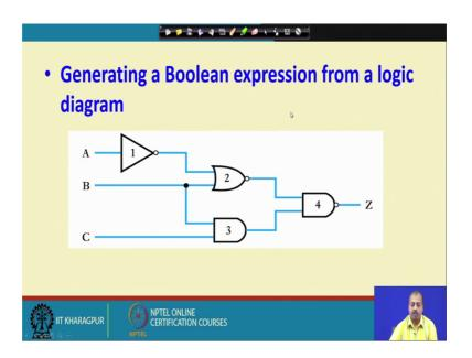
So, we can also do something for generating the Boolean expression from a logic diagram. So, suppose this is a Boolean this is a logic diagram. So, we can trace through this logic diagram to see how the corresponding Boolean expression can be derived.
