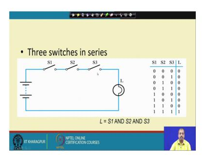
We can connect three switches in series like S 1, S 2, S 3. So, what happens is that here this lamp L get is current, only when all the three switches are closed. So, this can be represented in the form of a truth table, where this S 1, S 2, S 3 is so, if I just write down all the possibility. So, S 1, S 2, S 3 these are three variables so, it can start from 0 0 0 0 1 and go up to 1 1 1, where 0 means the switch is open and one means the switch is closed.
