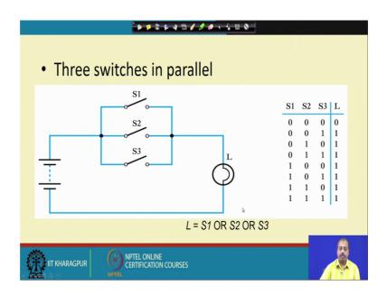
Similarly, we can have OR operation. So, we can have in parallel the switches may be connected in parallel S 1, S 2, S 3, they are connected in parallel so, whenever any of these switches are closed the lamp is turned on and, when all the switches are open and then the lamp is off. So, whenever this lamp L equal to 0 only when S 1, S 2, S 3 all of them are equal to 0. Otherwise whenever the any of them is equal to 1, the L value is equal to 1.
