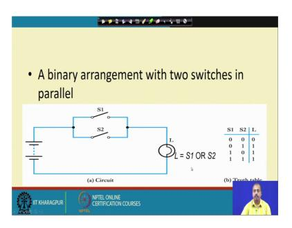
Similarly we can connect the two switches in parallel. So, apparently it seems why should we connect two switches in parallel, but for the sake of examples. So, let us take it like this that we have got two switches connected in parallel S 1 and S 2. And either of the switches being closed the light gets the lamp L gets current as a result it turns on. So, we can say that if again the same thing, if 0 for switches represent they are open and one represent they are closed.
