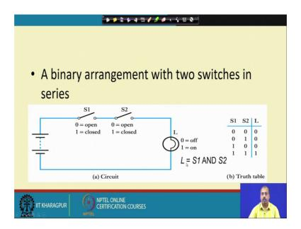
So, if we consider two switches like the suppose I have got S 1 and S 2 2 switch switches they are connected in series. So, the S 1 can be either open, or closed and S to can also be open or closed. Now, this lamp it get is the current flow only when both S 1 and S 2 are in closed state ok.
