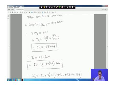
Now, total core loss is given 1500 watt. Core loss per phase 500 watt that therefore, core loss we can write V into I is equal to 500. So, I i the core loss component of the current 500 by V, so 500 by 288.7, so 1.73 ampere therefore, I 0 is equal to I i plus I m, so it will be 1.73 minus j 36 ampere right.
