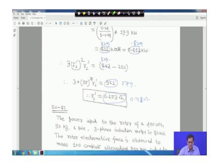
Therefore here your 3 I 2 dash square r 2 will be 829 minus 250 because that you have to make it, because that will be your actually rotor copper loss. So that means, 3 into 35 square into r 2 dash equal to 579 right. Therefore r 2 dash will be 0.158 ohm this blue ink one you see right this is the correct answer.
