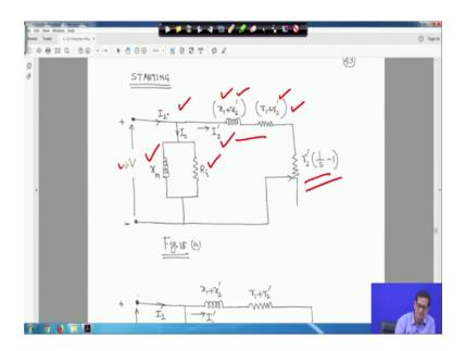
But this circuit if you look into this circuit right this circuit actually we have brought this magnetising component and the (Refer Time: 00:25) loss component just at the where at the beginning right. After that we are just for the simplification, but this kind of if you assume this kind of circuit, it will give it will not give accurate result whereas, result will be your calculation will be inaccurate
