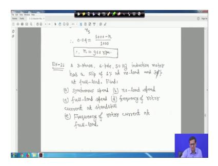
Similarly, example 2 is a 3 phase, 6 pole, 50 hertz induction motor has a slip of 1 percent at no load and 3 percent of full load right. Find the a synchronous speed, b no load speed, c - full load speed, d frequency of rotor current at standstill, and e - frequency of rotor current at full load right.
