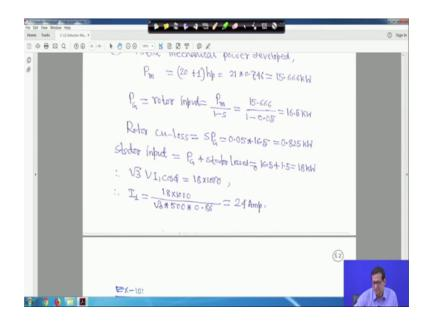
Rotor copper loss will be S P G, so S we know, P G we know. So, it will be 0.825 kilo watt right. So, because S is equal to 0.05, and stator input is equal to P G plus stator losses. So, P G is 16.5 and stator loss is 1.5, so it is 18 kilo watt right. And root 3 V I 1 cos phi is equal to 18 kilo watt.
