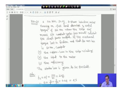
So, frequency of rotor current at full load f 2 is equal to S f l f. So, at full rotor S f l is 0.03 and this is 50, so it will be 1.5 hertz right. So, example 3 so a next one is a 6 pole, 50 hertz, 3 phase induction motor running on full load develops a useful torque of 160
