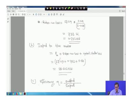
So, rotor copper loss will be 17.09 then your your that P m is equal to 17.09 is 0.04 by 1 minus 0.04. so it is coming 0.712 kilo watt. Now input to the motor input to the motor mechanical power output plus the rotor couple loss plus the total stator loss. Total stator loss is given actually 800 watt because in the problem it is given the total stator loss is equal to 800 watt here it is given 800 watt right.
