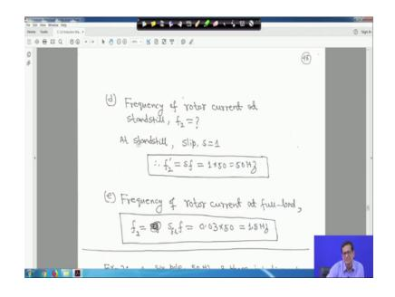
Now, frequency of rotor current at standstill, so f 2 is equal to how much? At stand still your S; S is equal to 1. So, naturally the rotor frequency the current frequency will 50 hertz your at standstill S is equal to 1, then that rotary stationary at that time at when rotor is stationary slip is 1.
