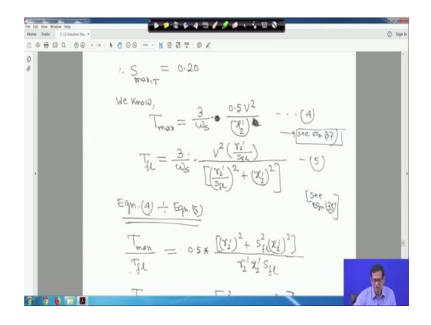
If you solve this one you will get S max is equal to 0.2 because other value is not feasible right. So, from S and you know that torque expression T max is equal to 3 upon omega S 0.5 V square upon x 2 dash here it is in detail c equation 37 right here it is in detail. So, here then; that means, you will get T full load torque is equal to 3 upon omega S into this expression here it is in detail from equation 35 right. So, all you have to keep it mind little bit you have to keep it in mind.
