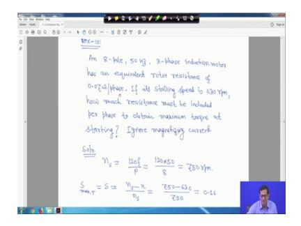
So, an 8 pole, 50 hertz, 3 phase induction motor has an equivalent rotor resistance of 0.07 ohm per phase. If its stalling speed is 630 rpm, how much resistance must be included per to obtain maximum torque at starting? Ignore magnetizing current right. So, n S is equal to you know 120 f by P, so in this case it is 8 pole machine right.
