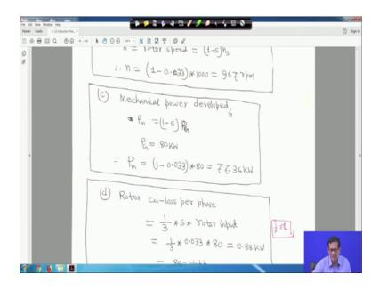
Now, next is mechanical power developed P m is equal to 1 minus S into P G. So, P m is equal to 80 kilo watt, so P m is equal to 1 minus 0.033 into 80, so 77.36 kilo watt right. Next is rotor copper loss per phase, so per phase that is one-third into slip into rotor input, so it is one-third into slip into 8. So, it will become 88 watt that is 0.88 kilo watt right.
