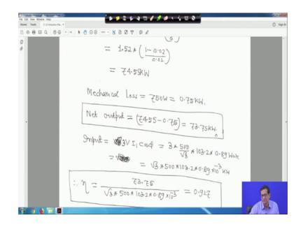
So, this is your into 1 minus 0.02 upon 0.02 slip is 0.02, so 74.5 kilo watt right. Now mechanical loss is equal to 70 750 watt it is given mechanical loss is given. Therefore, net output will be this 1 minus this 1 is equal to 73.75 kilo watt right.
