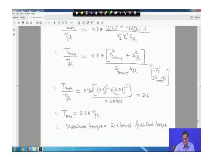
Now, that you put S max to you got 0.2 full load slip you know 0.04. So, it is a function of slip only and if you simplify it will be 2.6; that means, maximum torque will be 2.6 times the full load torque right. So, maximum torque 2.6 times the full load torque little bit practice is necessary right.
