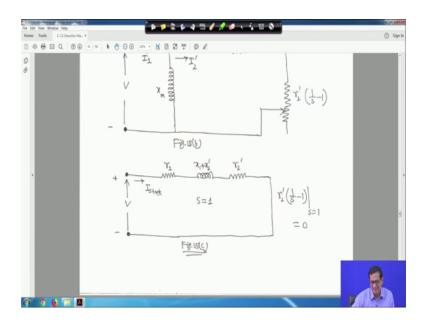
So, it is I starting S is equal to your 1, and this is r 1 right and this is x 1 plus x 2 dash this is r 2 dash and r 2 dash 1 upon S minus 1 S S is equal to 1, So this part is 0. So, at start this load at start S is equal to 1, so this part will be 0 right in that case this is here where I starting when S is equal to 1.
