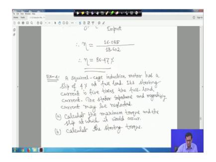
Next is a squirrel cage induction motor has a slip of 4 percent at full load. The starting current is five times the full load current the stator impedance and magnetizing current may be neglected. Even neglecting calculates the maximum torque and the slip at which it would occur and calculate the starting torque these two things right.
