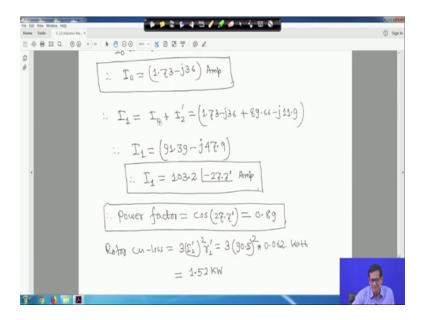
Therefore I 1 is equal to I 0, I 0 plus I 2 dash you see the circuit. If you add these it will be I 1 is equal to 103.2 angle minus 27.7 degree ampere. Now, power factor will be then cosine of 27.7.89 because voltage angle is therefore, taken as 0 and this is the stator
