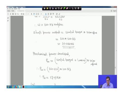
Now mechanical part developed is equal to P m is equal to useful torque plus losses into rotor speed, so useful torque is 160 and this loss is given 10. So, 160 plus 10 Newton metre into the rotor speed 100.53; so that is P m is equal to 17.09 kilo watt.
