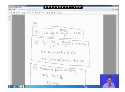
So, in this case solution is equal to it is given S is equal to f 2 upon f. Because f 2 is equal to except, so it is f 2 is equal to 100 by 60 because it is making 100 cycles per minute, so 100 by 60 cycles per second divided by 50. So, S S is equal to 0.033 3.3 percent right, n S is equal to 120 f by P. So, it is as usual 1000 rpm putting all these data n is equal to rotor speed is equal to 1 minus S n, so 1 minus 0.033 into 1000, so 967 rpm.
