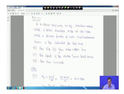
A 3 phase 500 volt, 50 hertz, induction motor with 6 poles develops 20 horse power at 950 rpm with a power facto of 0.86; total mechanical losses 1 hp that is 1 horse power. Calculate for this load, the slip, the rotor copper loss the you are the input if the stator losses total is 1500 watt the line current right, this you have to make it. Whenever you
