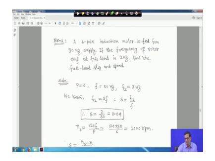
So, now take the example one. Suppose a 6 pole induction motor is fed from 50 hertz supply. If the frequency of rotor e m f at full load is 2 hertz right that is f 2 is equal to S f right. Find the full load slip and speed.
