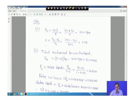
Now, we know that n S is equal to 120 f by P. So a 1000 rpm it is coming as usual and S is equal to you knowing this formula, so from this you are getting 0.05 right. So, total mechanical power developed will be 20 plus this one you have to add right h p, so 21.1 h p is equal to 0.746 kilo watt. So, it is 15.666 kilo watt right, so P G is equal to rotor input is equal to P m upon 1 minus S this is you know. So, put P m, put S here you will get 16.5 kilo watt right.
