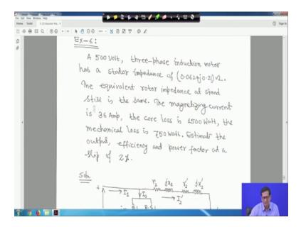
Next is example 6; a 500 volt, 3 phase induction motor has a stator impedance of this much. The equivalent rotor impedance at stand still is the same right. The stand still means when the slip is equal to 1, the magnetizing current is 36 ampere. The core loss
