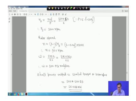
Now, n S is equal to 120 f by P; P is 6, f is 50, so n S is equal to 1000 rpm. Now rotor speed n is equal to 1 minus S into n S, so 1 minus 0.04 into 1000, so 960 rpm. Therefore, omega is equal to 2 pi n by because we need torque, so omega we require 2 pi n by 60. So, it is coming 100.53 radian per second right.
