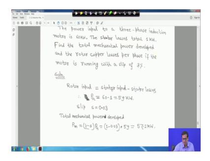
So, rotor input is equal to stator input minus stator losses in the beginning of the air gap power at that time I told you. So, it will be P G will be 60 minus 1 59 kilo watt and slip is 0.03. So, total mechanical power develop P m this expression you have also derived 1 minus S into P G. So, you will get 57.2 kilo watt right.
