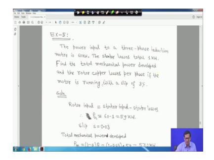
The power input to a 3 phase induction motor is 60 kilo watt. The stator losses total 1 kilowatt. Find the total mechanical power developed and the rotor copper losses per phase, if the motor is running with a slip of 3 percent right.
