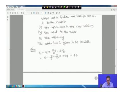
So, actually this f 2 is equal to S f is equal to this is given 120 complete cycles per minute. So, rotor frequency 120 by 60 right, so how many cycles per second actually that is actually 2 hertz cycles per second, so it is 2 hertz right. Now S is equal to then 2 upon f because S f is equal to 2, so S is equal to 2 by 50, so 4 percent, 0.04 right.
