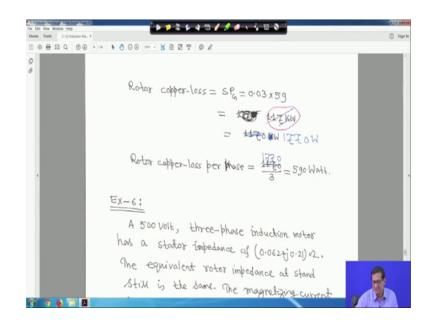
Now, rotor copper loss we also derived this formula S into P G. So, it is 0.03 into 59. So, it is actually your 1 11770 watt right this calculation this blue ink you see that 1770 watt right. So, rotor copper loss per phase divided by 3 it will be 590 watt is a simple problem only you have to keep it some formula in your mind right.
