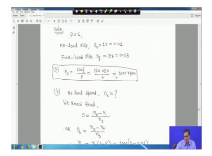
So, when P is equal to 6 no load slip given that is 0.01, full load sleep is given that is 0.033 percent, so n S physical 120 f by P. So, it is 1000 rpm substitute all these value it is 120; f is equal to 50 hertz and P is equal to 6 poles, so 1000 rpm do not make it p r right, then you will make a mistake here is number of poles right, so 1000 rpm.
