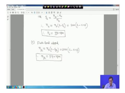
Now c is the full load speed, so n f l you can just replace this suffix 0 by f l; n f l is equal to n S 1 minus S f l this is your 1000 and S f l is 0.03. So, it is coming 970 rpm right.
