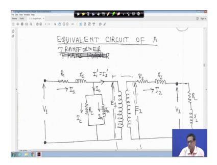
Now, equivalent circuit of a transformer because we have seen transformer, but we have to obtain the equivalent circuit of transformer because you have to solve problem how to solve the problem for an equivalent transformer or a equivalent transformer. For that we need to know the equivalent circuit of a transformer, right.
