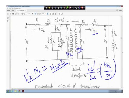
And current here is I 2 dash therefore, you can make it I 2 dash into N 1 that is mmf of the primary side is equal to mmf of the secondary side that is N 2 into your N 2 into your I 2, right. So, this is I 2 and at this N 2. So, N 2 I 2 is equal to how to I 2 dash N 1, right.
