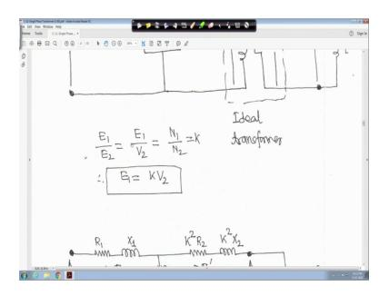
If it is so, similar way if it is so, then if you look into this that E 1 by E 2 is equal to you know N 1 by N 2 and E 2 is equal to V 2. So, E 1 by V 2 is equal to your K therefore, E 1 is equal to K into V 2.
