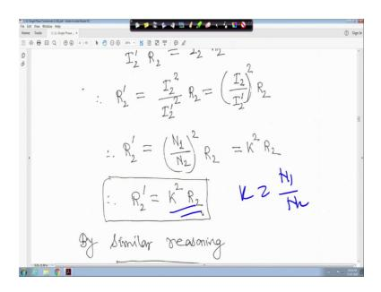
But we have seen earlier that K is equal to we have seen earlier the K trans ratio is equal to N 1 upon N 2 therefore, R 2 dash will be K square into R 2, right.
