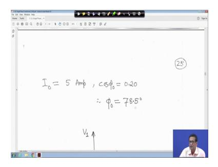
Now, I 0 is given 5 ampere and cos phi 0 is 0.2 is given. So, phi 0 is equal to 78.5 degree.
