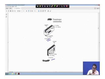
Next is the little bit of construction of the transformer. So, this is I have taken from a book, right. So, generally that whatever we solved the numericals and other thing that is but very equivalent circuit. But if you look into that that lower that is this is core this is core type transformer that low voltage winding an above that your high voltage winding how they are there and this is laminated core. That is your real that is your practical transformer.
