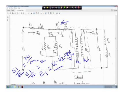
That means this side that means, this side voltage transformation it will be K into V 2 because it is ideal transfer this trans ratio is N 1 this is N 2 E 1 upon E 2 is equal to N 1 upon N 2 that is your E 1 upon E 2 is equal to your N 1 upon N 2, right. But E 2 is equal to V 2 because this thing is transformed to this side, right E 2 is equal to V 2 that means,
