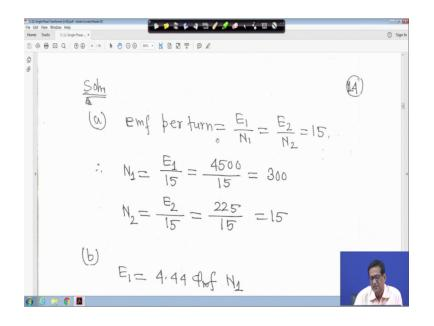
So, emf per turn is equal to E 1 upon N 1 is equal to E 2 by N 2 is equal to 15, it is given therefore, N 1 is equal to E 1 upon 15 that is also V 1 up on E 1. So, right is equal to E 2 upon N 2 is equal to 15 that way you can make it. So, it is given 4500 by 15. So, you will get it is 300 because it is primary side where 4500 volt. Similarly secondary side 225 Volt so; N 2 is equal to 225 by 15, so it is 15, right N 2 is 15.
