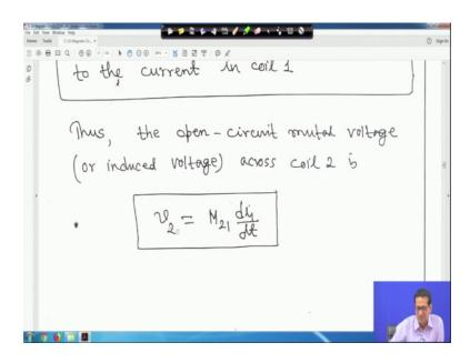
So, thus the open circuit mutual voltage or induced voltage right across coil 2 will be v 2 is equal to M 2 1 d i1 upon d t because, flux i1 actually creating your current i1 actually creating the flux i1 and part of the flux linking the your coil 2, therefore v 2 will be M 2 1 d i1 upon d t that there it is right. So, v 2 is equal to N 2 1 d i1 upon d t it is a in your induced voltage right due to the flux main thing the other coil.
