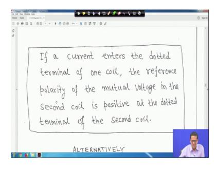
If a current enters the dotted terminal of one coil, the reference polarity of the mutual voltage in the second coil is positive at the dotted terminal of the second coil, this is the language I have written that you will come to that figure and other thing. If a current enters the dotted terminal of one coil, the reference polarity of the mutual voltage right in the second coil is positive at the dotted terminal of the second coil.
