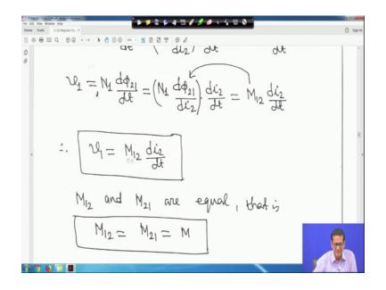
But, M 1 2 and M 1 2 are equal that is M 1 2 is equal to M 2 1 is equal to M it cannot be different right, this way have that way mutual inductance has to be same right. So, M is actually M 1 2 is equal to M 2 1 right. So, this is your equation number I did not put just make step by step understandable to you right.
