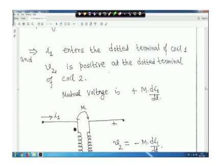
Now, similarly now that is I that is i1 enters the dotted terminal of coil 1. So, i1 actually entering into the dot so, this i1 actually entering into the dotted terminal right much more we will see. So, and v 2 is the positive at the dotted terminal coil 2 therefore, mutual voltage is plus M d I d i1 upon d t. This is our reference polarity you have taken this is a reference polarity you have taken plus.
