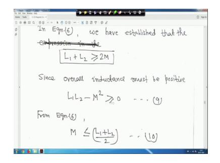
So, that is what is written in right. So, equation 6 we have established that L 1 plus L 2 greater than equal to 2 M; that means, M and here for since overall inductor that is for series circuit; you have seen series circuit L 1 plus L 2 greater than equal to 2 M and the overall inductance must be positive, if L 1 minus a your L 1 L 2 minus M square greater than 0 right.
