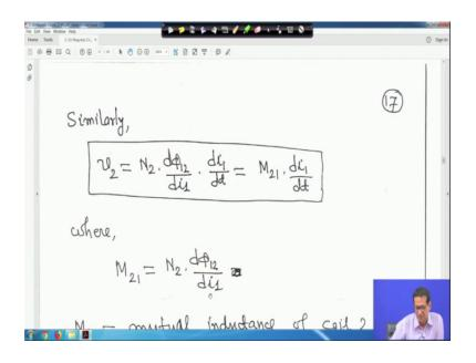
Now, similarly for v 2 case ; v 2 case we can write again chain rule v 2 is equal to N 2 d phi 1 2 upon d i1 into d i1 upon d t this actually it is actually mutual inductance. So, N 2 d phi 1 2 upon d i1 we are writing N 2 1 d i1 upon d t where, M 2 1 is equal to N 2 your what you call N 2 into d phi 1 d phi 1 2 upon d i1 this is actually mutual inductance right.
