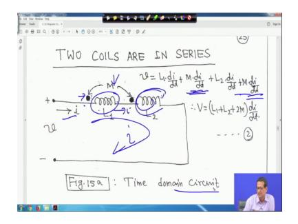
So, now 2 coils are in series; if 2 coils are in series how it looks like look in this case only how to write the equation in this case the current I because it is series 2 coils are they look. Here in the take this 1st coil is dot current is entering into the dot in the 2nd coil also same current i is entering into the dot; that means, sign should be plus this is L 1 L 2 their inductances. So, clear i1 entering the dot all this is one coil is dot is marked here.
