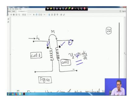
Suppose this your what you call this current your what you call in figure 10, the 2 coils are there dot are shown this dots are shown. Here current i1 is entering and mutual inductance between this coil is shown by M here it is M a mutual inductance and this is coiled to should be written M into d i1 by d t because, current is i1 and mutual voltage
