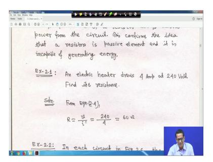
So, find it is resistance so, we know R is equal to v is equal to iR. So, R is equal to v by i v is equal to 240 and i is equal to 4 so, 60 ohm the resistance, right.
