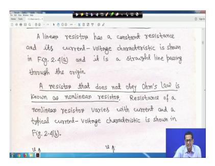
So, a linear resistor has a constant resistance, and its current voltage characteristic is linear right as shown in passing through the origin.
