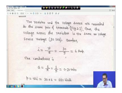
So, current will be i is equal to v by R is equal to 30 by 5 is equal to 6 ampere.
