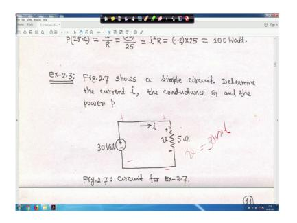
So, in this so, all this cases, you can see it is 8 watt thousand watt or 100 watt all the cases resistor actually absorbing power, right this is, this is another small thing that figure 2.7 shows simple circuit than the current i the conductance G and the power p. So, it is 30-volt source, and here one resistor is there and it is 5-ohm resistance and current flowing through this your is i, right.
