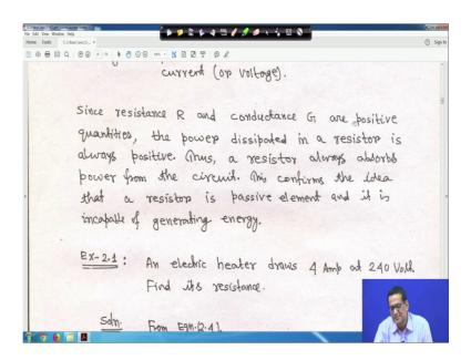
So, since resistance R and conductance G are just what I will told, that it is positive right quantities the power dissipated in a resistor is always positive. I told you thus a resistor always your absorbed power from the circuit it absorbed, right this confirms the idea that a resistor is passive element. And it is incapable of generating energy, this is very important for you. When we will listen this video, right just see that what; what we are discussing, right.
