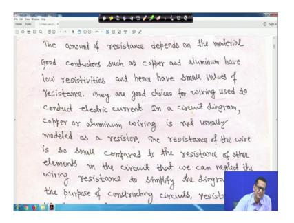
So, in circuit connection copper or aluminum is not usually modeled as a resistor, you will take resistance of the wire in the if you take resistance of wire is 0, right. So, the resistance of the wire is so small compared to the resistance of the other elements in the circuit that we can neglect the wiring resistance.
