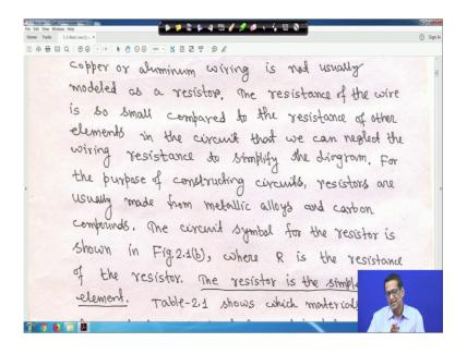
So, in the first year when we will first year when we will do first year lab, there you will see barrier type of rheostat, right. So, the circuit symbol for the resistor is given this is this is the circuit symbol for the resistor is given here and I told you something about these also why you will make it like this, right. So, and there are some materials of I have wrote it for you the resistivity for commonly use material like gold.
