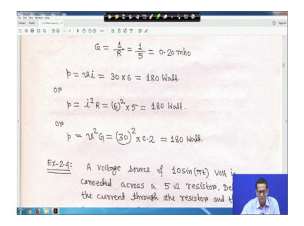
So, conductance is G is equal to 1 upon R. So, 1 by 5 so, 0.2 mho, because reciprocal about. So, power is equal to v into i is equal to 30 into 6. So, 180 watt this we can calculate, or p is equal to i square R that is 6 square i is the i is 6 ampere, we have calculated this 6 ampere 6 square into 5.
