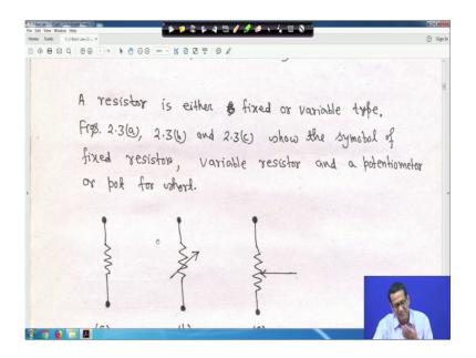
Now, 3 you have to understand each and everything as symbol also. So, a resistor is either a it may be either a fixed resistor or a variable type, right. So, there are 3 different symbols are shown, this is actually this is fixed type this is 2 terminals are there. So, this is a fixed resistance R. Say right this is a fixed resistance.
