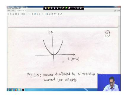
So, it is graph will be either this side you plot i or v, this is power it is a parabolic function just I have drawn right.
