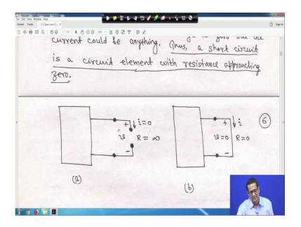
So, for example, look at this circuit before explanation suppose this is a this is an this is a your what you call some electric circuit represented by your just a simple box, right. And this is open, so that means, R is equal to infinity; that means, current is 0. So, when R is equal to infinity or R tends to infinity i is equal to v by R so, if R tends to infinity I will be 0. So, it is called when R tends to infinity means is says it is an open circuit, right?.
