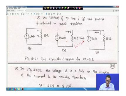
So, this is actually G is equal to 0.1 mho conductance is given of the circuit, right. So, so, in this case a voltage is given your 100, 100-volt that is 100 volt. So, you have to find out that what is the current. So, just let me let me clean this one, right?
