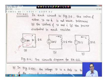
Another small example in each circuit in figure 2.6, right; so, this is 3 circuits are there the value of either v or i is not known. Ri we have to find determine the a the values of v and i b the power dissipated in each resistor. So, you have to find out v or i v or i right whatever it is known are unknown, unknown quantities you have to find out.
