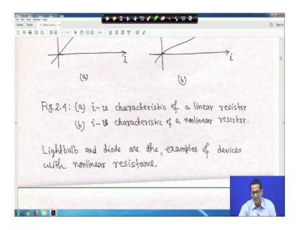
For example, your light bulb and diode are the examples of devices with non-linear resistance.
