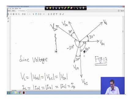
I mean from this phasor diagram, again I have to go on top right just hold on here, here from this phasor diagram. With respect to that this is angle 30 degree, with respect to V an it is ninety degree and with respect to V an this is your minus 210 degree right. So, so, that is your what you call that your V ab, V bc and V ca right.
