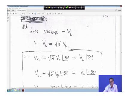
You do it yourself, right other phasor diagram. So line voltage is equal to V L and we know V L is equal to root 3 in to phase voltage right magnitude.
