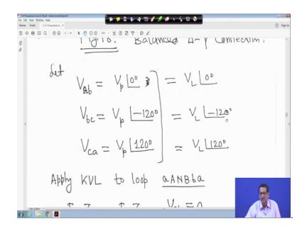
So, that means, V ab is equal to same thing we have done V p angle 0 degree, V bc V p angle minus 120 degree and V ca is equal to V p angle 120 degree. So, V L angle 0 degree, V L angle minus 120 degree V L angle 12[0]
