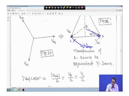
So, it is in this direction V an, that means, this is my say just as a reference am putting, this is V an, if i make it right because this is this direction, so V an will lag from V b by minus 30 degree So, that is why that is why your V an is equal to V L upon root 3 angle minus 50. So, V p upon root 3 angle minus 30 degree.
