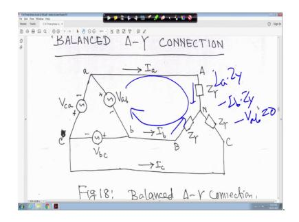
So, if you apply your K KM lining this one if you apply your you this here if you apply KVL here, if you apply KVL here, it will be I a into Z y right. So and current this is I a flowing this, but this current is going this way. So, it will be minus I b into Z y and it is encountering minus tabular first, so minus ab is equal to 0 right.
