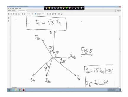
So, line current earlier we saw star connection your line will your what you call your line voltage is equal to root 3 line phase voltage and for delta connector, volt line current is equal to your what you call going to that that is, your root 3 times phase current. So, I LL is equal to root 3 times phase current right.
