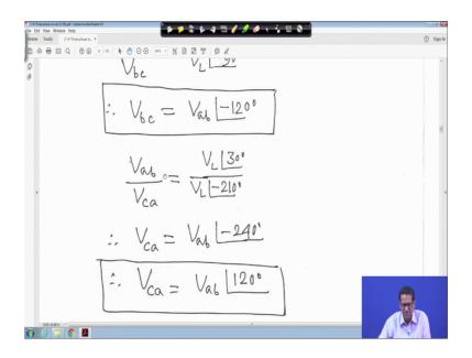
Now, if you make divide V ab by V bc, if you make V ab by V bc, it is V L angle 30 by V L angle minus 90 therefore, V bc is equal to, it is it will go up it will be 120 degree, so V bc is equal to V ab minus 120 degree right. Similarly V ab upon V ca if you make, you
