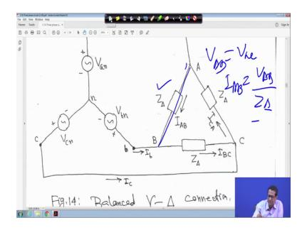
Now, I AB is equal to V AB upon Z delta because, this is my circuit; that means, this voltage your this voltage right that your V AB that is my V AB, this voltage A to B and is equal to V ab right, same voltage impedance and this is my Z delta I AB. So, I AB is equal to V AB upon Z delta right, for this phase right. So, same thing here, we are writing same thing we are writing I AB is equal V AB upon Z delta, I BC is equal to V BC upon Z delta, I CA is equal to V CA upon Z delta all right.
