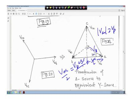
So, that means, this one this V ab right, V ab this is actually this portion actually V ab by 2 it is half it is equilateral triangle. So, V ab by 2 is equal to this is V an, this is actually V p right because, this is the magnitude V an, so this is V an is equal to V p right. So, it is V p then, cos 30 degree right here is equal to is equal to V p cos 30 degree right.
