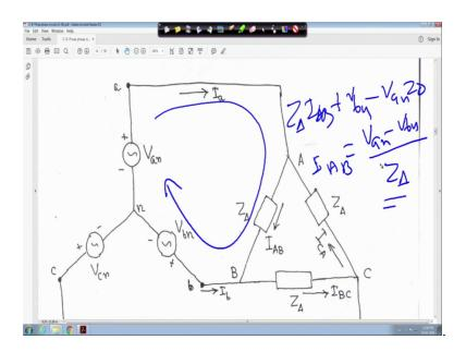
So, now another way to get this phase current is to apply KVL, for example, applying KVL around loop, so, aABbna right.
