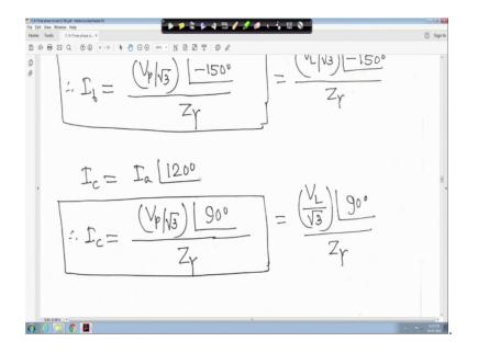
Similarly, I c is equal to one angle I your 20 degree you put I a is equal to here you will get V p upon root 3 angle Z divided by Z y and angle 90 degree.
