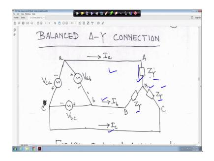
So, in this case your what we call that source is delta, but load is star. So, when loading this star in this case, line current is equal to phase current because same current is your what we call, the same current i is going entering here right. So, line current is equal to your phase current right so, but e your what you call this is voltage source, your what we call and this is at your delta source is delta.
