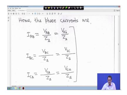
So, hence the phase currents are simply I AB is equal to V AB upon Z delta, if you come to the circuit if you come to this circuit A AB is equal to V ab upon Z delta right here. So similarly your, I BC and I CA this is I BC, V BC upon Z delta I CA is equal to V CA upon Z delta right.
