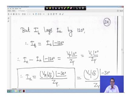
But I a lags I b by 120 degree, we know that, but I b lags 120 degree, simply substitute I b is equal to I a minus 120 degree, you put it here and you simplify, if you simplify you will get, I a is equal to V p upon root 3 divided by angle minus 30 degree by Z y.
