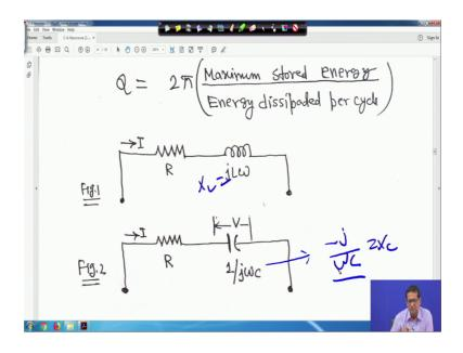
So, quality factor sometimes for a circuit is defined by 2 pi into maximum stored energy divided by energy dissipated per cycle right. So, for example, it is called quality factor right of the coils capacitors and circuit. So, in general Q is equal to 2 pi into maximum stored energy divided by energy dissipated per by your what you call per cycle. Now for
