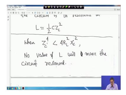
The circuit is in resonance at 1 is equal to half C ZC square, I mean if ZC to the power 4 is equal to 4 RL square XC square means this term will be 0 so; that means, L will be half C into ZC square right. So; that means, the circuit is in resonance at L is equal to half C ZC square and when ZC to the power 4 is less than 4 RL square XL square no value L will make the circuit resonant. So, if this condition is there; that means, under
