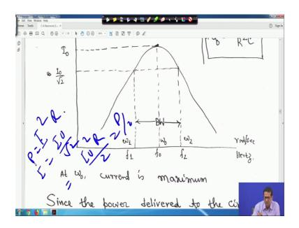
So, power delivered to the circuit the power is 1 half of the maximum value which occurs at omega 0 right therefore,; that means, whatever resonance at resonance power is I 0 say R I I square R is equal to if I is equal to I 0 then I 0 square R, but at I is equal to I 0 by root 2 it will be half right. So, the points corresponding to omega 1 and omega called the half power points.
