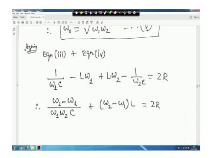
So, if you do so and simplify you add and simplify you will get omega 2 minus omega 1 upon omega 1 omega 2 C plus omega 2 minus omega 1 L is equal to 2 R right.
