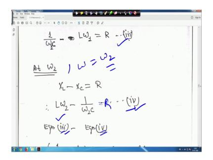
So, this is equation 4 and this is equal to R actually right. So, now what you do subtract equation 4 from equation 3, I mean this equation you subtract from this equation if you do.
