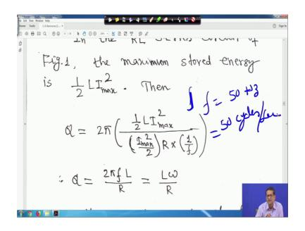
Whenever we say whenever we say f is equal to f is equal to 50 hertz; that means, it is 50 cycles per second right. So, it is per cycle, so it is divided by f right. So, if you after simplification after simplification simply you will get Q is equal to 2 pi f L upon R that is your L omega by that is your L omega by R right.
