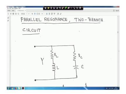
We have taken a simple two branch circuit right. So, your this is R L over L that is one inductive branch and this is one capacitive branch right. So, it is R L L omega and it is RC your XC right. So, this is you have to see the parallel resonance of the circuit. So, Y is the admittance right. So, Y is equal to your Y is equal to that admittance is equal to Y L plus Y C right.
