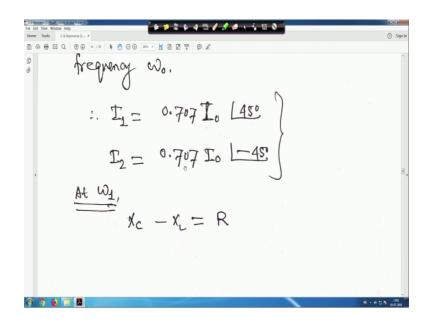
So, this one therefore, I 1 is equal to 0.707 angle I 0 angle 45 degree similarly I 2 is equal I 0.707 angle minus 45 degree, but at omega 1 at omega is equal to omega 1 XC minus XL is equal to R right.
