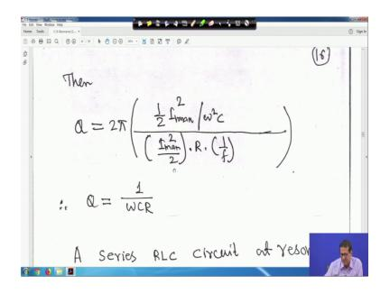
So, this in that case for in the case of capacitor; so, 2 pi half I max square upon omega square C divided by same thing I max square by 2 into R into 1 upon f right. So, if you do, so Q will become one upon omega C R right; that means, this for quality factor for inductive circuit is Q is equal to L omega by R and for capacitive circuit it is Q is equal to 1 upon omega C R right.
