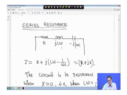
So, in the case of series your simple RLC circuit are j L omega minus j upon omega C right. So, Z is equal to impedance Z is equal to R Plus j L omega minus omega C is equal to you can right say R Plus jX in this form right.
