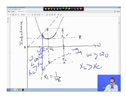
So, X C is equal to 1 upon omega C looks like a rectangular hyperbola right. So, that this dash line is plot right. So, this thing from here to here, from here to here right, from here to here this is my X L and from here to here this is an X C. And at X L is equal to X C that is frequency is equal to this 1 omega 0 right.
