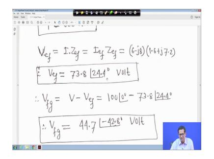
So, this is your 73.8 and angle 24.4 degree volt. Similarly, V fg is equal to v minus V ef you apply kvl here right, then you will get 0 here what we call V fg we apply the kvl in the circuit. So, am not going to the circuit again and again just you draw and look it you have done this circuit everything, only consider instantaneous polarity and solve it. So, it will be 100 angle 0 ohm minus 73. angle 24.4 degree. So, this is coming actually 44.7 and angle minus 42.8 degree volt right.
