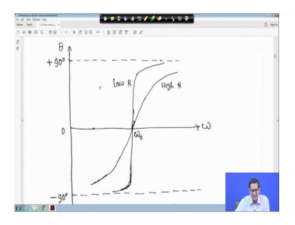
So, for very small resistance this is your omega and this is theta. Theta versus omega curve for small resistance the plot is very sharp look at that and for high resistance this is the plot and this is my omega 0. This side is plus 90 degree, this side is minus 90 degree right.
