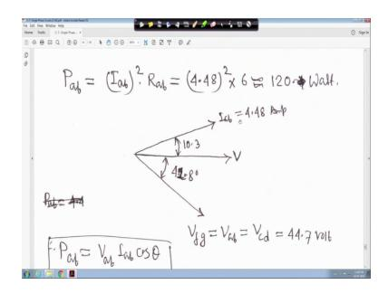
So, at P ab power loss is equal to I ab square R ab. So, it is I ab is equal to 4.48 square and R ab is equal to 6 so, it is 120 watt right.
