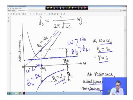
So, if you plot now admittance versus omega same as your what you call now I will do impedance versus omega for series admittance circuit. For parallel, we are plotting admittance versus omega.
