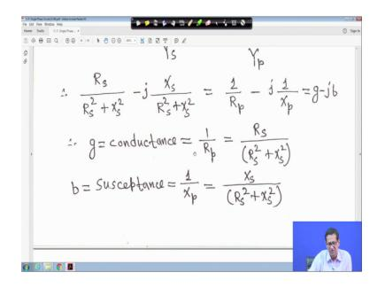
G is equal to conductance is equal to 1 upon R p. So, 1 upon R p is equal to separate real and imaginary part, 1 upon R p is equal to R S upon R S square plus X S square this one right. And similarly your 1 upon X p is equal to X S upon R S square plus X S square this is 1 upon X or just go right, R p is equal to R S square plus X S square upon R S, X p is equal to R S square plus X S square upon R S, X p is equal to R S square plus X S square upon your X S right.
