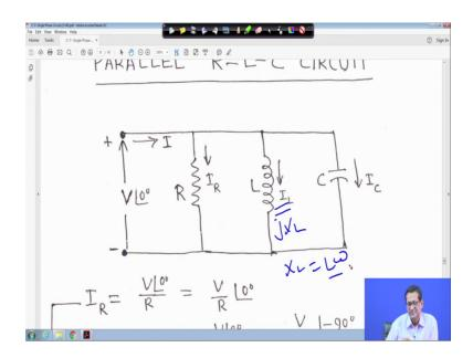
So, now this is a simple parallel circuit right RLC circuit, voltage source V is given, R, L and C, all these things are parallel. So, current flowing through this R is I R, through L, I L and through I C right. So, what we have to do is that is a parallel circuit. So, let us see I R, I L, I C and I, this total current is I, I is equal to I R plus I L plus I C right kcl if you apply here.
