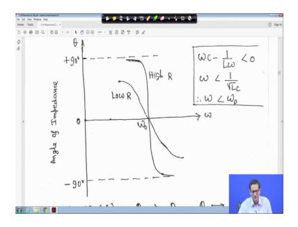
Now, if you plot this one, this is same as before this is angle of a impedance plus 90 degree, this is minus 90 degree right. So, this is very high value of R this is the plot and for low R this is the plot and this is my omega 0. The way we explain the previous one
