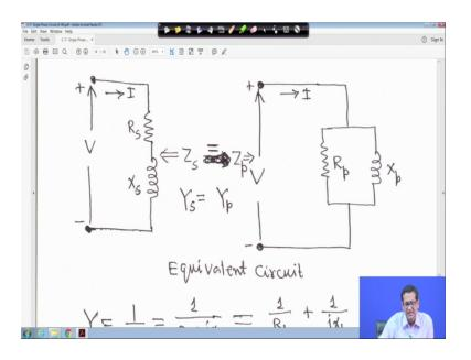
For example this is my series impedance R S and X S and this is my supply voltage V. Now, question is that we want this one is equivalent R P and X P these 2 circuits are equivalent to each other right. That means, Y S is equal to Y P; that means, series admittance is equal to parallel admittance and this branch is R P and X P.
