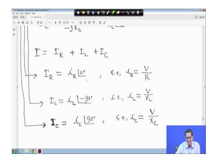
So, IR is equal so, i R angle 0 because, your resistive circuit this is your circuit and this is your this is your what we call V upon R angle 0. So, IR is equal to your i R angle 0 that is i R is equal to V upon R, IL is equal to i L angle minus 90 degree. This i L is nothing, but V upon X L this is the magnitude. Similarly, IC is equal to i C angle 90 degree, i C is nothing, but V upon X C right.
