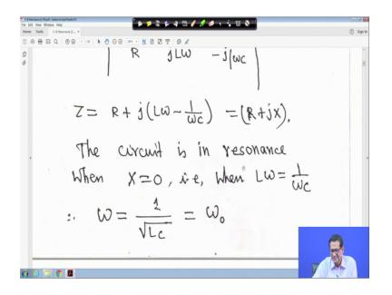
The circuit is in resonance when X is equal to 0 that is when X is equal to 0 means that L omega minus omega 1 upon omega C is equal to 0 means that L omega is equal to 1 upon omega C; that means, omega is equal to your 1 upon root over L C is equal to omega 0. This omega 0 we will call that your what we will call that is the resonance frequency omega 0 right.
