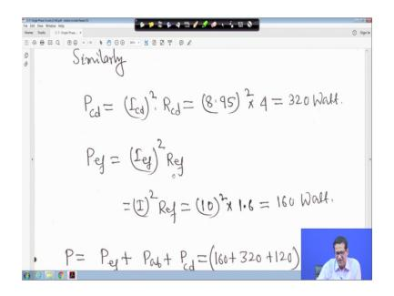
Similarly, your P cd is equal to I cd square R cd, it is 320 watt right and P ef, I ef square I ef square R ef so, it is coming out 160 watt. So, total P is equal to P ef plus P ab plus P cd it is 600 watt right.
