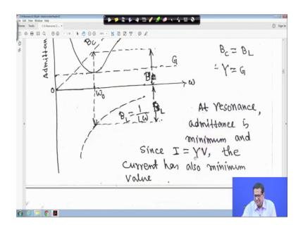
So, in this case and since I is equal to YV so, Y is that admittance the current has also minimum value for the parallel circuit right.
