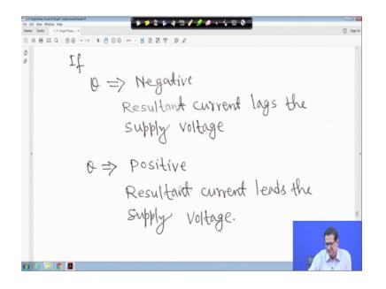
Theta negative then resultant current lags the supply voltage if theta is negative and if it is positive resultant current reach the supply voltage right.
