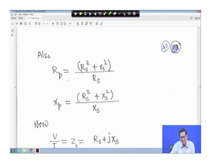
So; that means, this is that parallel your series one series impedance R S plus jX S can be represented by 2 parallel connecting a or what we call impedance. One is of course, is
