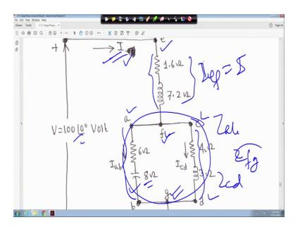
So, this circuit actually it is your this point you have to find out this is the current I and this point is a, this is b, this is c, this is d, this point is e, this is f and this point is g right.
