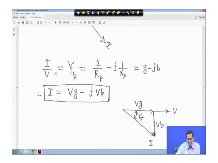
Similarly, for parallel equivalent I by V is equal to I P because, it is admittance that is why I by V and is equal to 1 upon R P minus j 1 upon X p is equal to g minus jb right. Therefore, my I is equal to you multiply I by V is equal to g minus jb therefore, I is equal to V g minus jV b.
