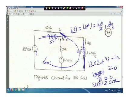
Because here, I mean when switch was in position a; so inductor is behaving across a short circuit and this is the voltage across the inductor. So and current through this is one ampere this is your i 0 i 0 minus is equal to i 0 plus right is equal to i 0 is equal to one ampere that you have seen.
