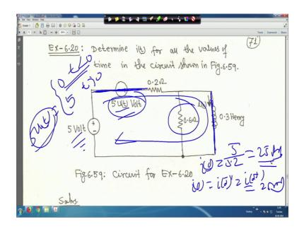
So, one thing is there that this is this 5 volt is connected, but this is 5 u t right. So, this is 5 u t means this is you know that 5 u t means it is 0 for t less than 0, and it is 5 for t greater than 0 because u t is 0 for t less than 0 and u t is 1 for t greater than 0 right.
