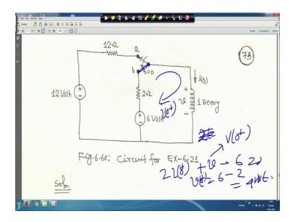
So, if switch is in position if switch is in position this one, at the just at the time of switching the current flowing through this is i 0 plus right. So, it will be if you move like this, it will be 2 into here I am writing it will be 2 then i then 0 plus right plus v minus 6 is equal to 0, but i 0 plus is equal to 1. So, v will be is equal to your actually it will be v 0 plus right v is equal to v 0 plus, it will be 6 minus 2 is equal to 4 volt right. So, let me clear it.
