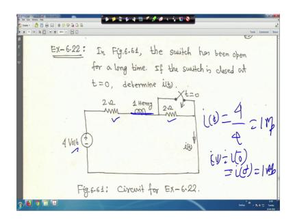
So, this switch was open for a long time means, that inductor is behaving like a short circuit right. And, it was opened for a long time that one you find out what is your i 0; and i 0 is equal to at the time of switching i 0 is equal to i 0 minus and at the time of switching i 0 plus it will not change right.
