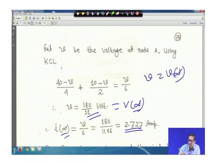
This v is nothing, but v infinity the steady state, when inductor is acting as a short circuit right. So, if you solve this v actually this is v infinity. So, it is 180 upon 11 volt right. So, in this case i infinity will be v by 6 because across that 6 ohm resistance your voltage your voltage this nodal analysis we got this v infinity.
