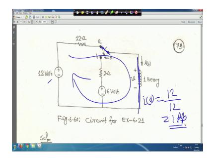
Suppose this one it was positioned like this for a long time, at that time inductor is behaving like a short circuit right and current through this that initial current that is i 0, it will be 12 volt and if you apply KVL here if you apply KVL here like this, it will be 12 by 12 volt by 12 ohm is equal to 1 ampere right. So, this is your i 0 is equal to i 0 minus is equal to i 0 plus that is your 1 ampere right. Now, at t is equal to 0, the switch has been thrown it here right.
