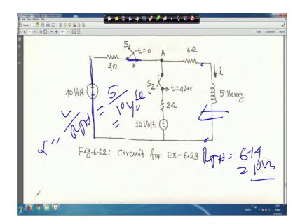
And R Thevenin will be is equal to we are looking from this terminal you are looking from this terminal, this is open it will be 6 plus 4 is equal to 10 ohm this is R Thevenin and tau is equal to L by R Thevenin right.
