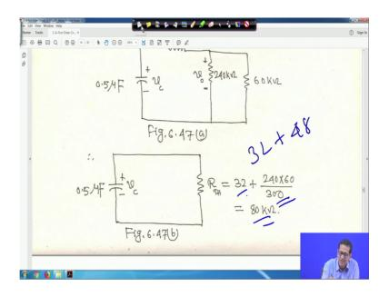
Now, at t 0 plus switch moves from A to B, that is your the switch actually moving from A to B and this is the circuit this 32 kilo ohm and 240 and 60 kilo ohm are in parallel right this 2 are in parallel. Now, as their equivalent will be that you are R Thevenin will be 32 plus 240 into 60 upon 240 plus 60 whatever it comes it is 80 kilo ohm, right and capacitor is 0; microfarad 5 microfarad. Therefore, tau is equal to C into R Thevenin. So, it is 0.04 second right.
