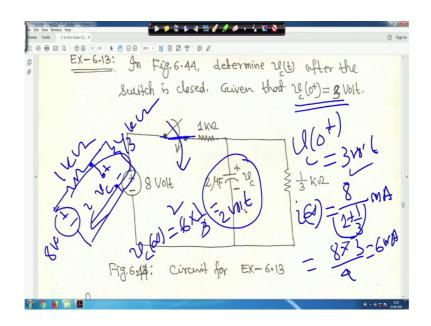
So, anyway come to the next problem. So, hope you are understanding this. So, this is actually you have to find out for this circuit, you have to find out that you are in your in this figure, you have to find out that your V C t. Determine V C t after the switch is closed right. So, switch is closed and initial value of V C 0 plus is given 3 volt it is given. V C 0 plus is equal to 3 volt, it is given. Now, switch is closed that means switch is closed right.
