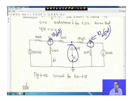
Similarly, this nodal analysis V 2, we have to apply it as V 2 infinity, right. So, that means, at steady state it is reached, switch was closed for long time. So, at this node, you apply for your nodal analysis KCL here also you apply for KCL. So, this we have studied much studied before. And so, many problems we have solved.
