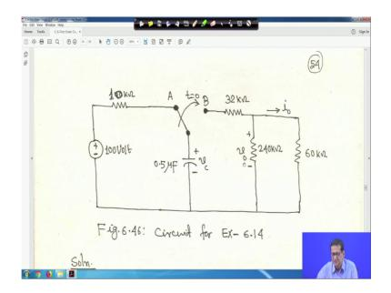
So, this is the circuit this was in position a for long time right at t is equal to 0 the switch moves instantaneously to position B determine V C t V 0 t i 0 t in part B the total energy dissipated in the 60 kilo ohm resistor right. So, the switch A this switch was in a position A for long time after that it move at t is equal to 0 it moves from A to B right. So, you have to find out V C t V 0 t i 0 t.
