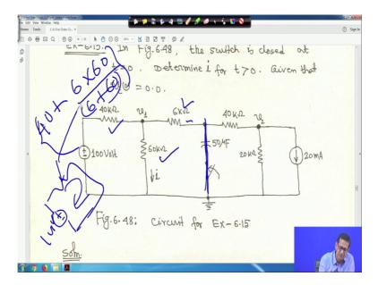
So, next, this one you take. In figure 48, the switch is closed at t is equal to 0. Determine i for t greater than 0 given that V C 0 is 0; that means, initially switch was open and
