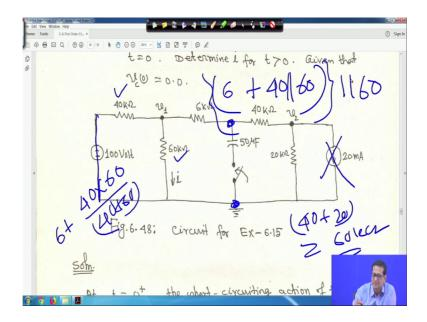
So, right hand side, it will be 40 plus 20; that is your 60 kilo ohm right. This is under because, this you want to find out R Thevenin. So, this should be gone this is open circuit. This is short circuit and this side as it is short circuit. So, 40 kilo ohm and 60 kilo ohm are in parallel with that 6 kilo ohm is in series; that means, left hand side, I mean this side, it will be your 6 plus 40 into 60 divided by 40 plus 60 right, this side.
