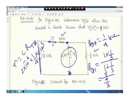
So, you will get R Thevenin right is equal to your 1 into 1 by 3; then, one this 1 kilo ohm and 1 3rd kilo ohm are in parallel, right, because, these are finding out from this point only so divided by 1 plus 1 by 3. So, it is 1 by 3 divided by 4 by 3, right. So, that is R Thevenin is equal to your 1 by 4 kilo ohm right and capacitor is 2 microfarad. So, time constant tau is equal to C R, R Thevenin, C R Thevenin.
