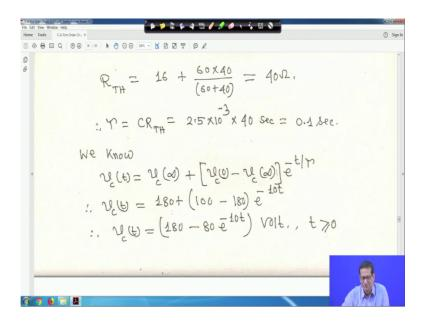
So, it is e to the power minus 10 t. So, it is V C t is equal to 180 minus 80 e to the power minus 10 t volt; that is t greater than equal to 0, right.
