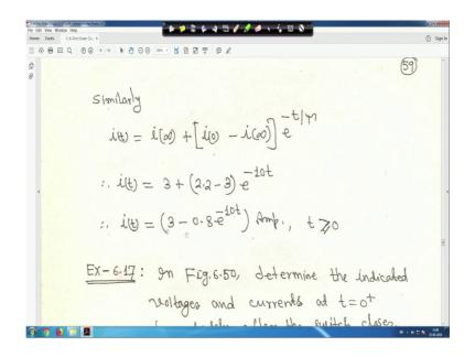
Similarly, for i t is equal to i infinity plus i 0 minus i infinity e to the power minus t by tau, right. So, i t is equal to 3 plus 2.2 minus 3 e to the power minus 10 t. So, i t is equal to 3 minus 0.8 e to the power minus 10 t ampere for t greater than 0 right. So, this are this is a you know little bit coming to this problem diagram, little bit you do it and just see that only that little bit understanding is required.
