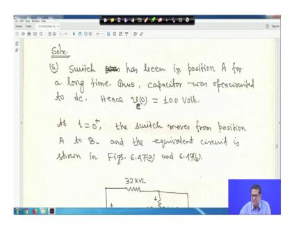
Switch has been in a position for long time the capacitor was open circuited DC as it was in the long position. So, capacitor here was open; I mean steady state for this part left hand side right.
