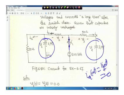
So, next one is next one is this is this is very interesting problem. So, figures 50 determine the indicated voltages and current at t is equal to 0 plus immediately after the
