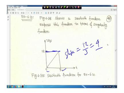
So, another one we will take thing this is like this figure it shows a sawtooth function, express this function in terms of singularity function, it is a sawtooth function is given right. So, it is basically a ramp function and your another thing is that is a gate function right. So, it is a slope it is this height, it is this height it is 12 right and this is from here to here it is 3. So, it is slope is equal to your 12 by 3 is equal to 4, the slope is equal to 4 for this straight line right.
