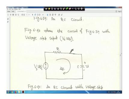
So, this circuit it this is the circuit and this can be represented as this is an RC circuit, this can be represented as that is V s u t that is; source voltage is this is your what you call this switch is closed. And it can be written as V s u t then R and C. Actually idea is simply like this for t less than 0 we know the unit step function for t less than 0 u t is equal to 0. And for t greater than 0 u t is equal to 1.
