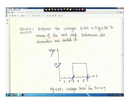
It is given that express the voltage pulse right in figure 35, this is figure 35, in terms of the unit step determines it is derivative and sketch it. So, it is looks like it is a gate function actually, it is a gate function. Actually at time t is equal to 3 second and actually idea is like this, this graph is like this. So, it is a voltage pulse so at time t is equal to 3 it is switched on and say time t is equal to 6, it is switched off right.
