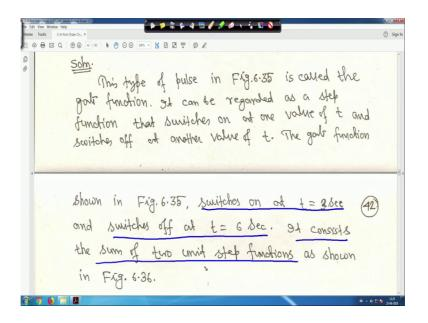
So, it is a gate function. So what I said? A t 3 second it is switches off and t 6 second at t is equal to your 3 second, it is switching on switches or switches on at t is equal to 3 second, h ere it is it is switches on at t equal to 3 second and switches off at t equal to 6 second; that means, it consists of sum of 2 unit step functions as shown in figure 36. So, let us see how is it?
