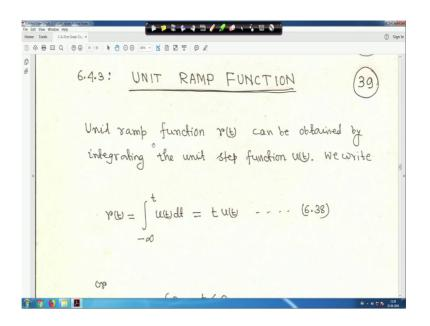
There are many other singularity function, but we will we will come up to ramp function some example. So, unit ramp function, in this case unit ramp function r t can be obtained by integrating the unit step function u t.
