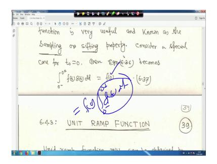
Now, therefore, consider a special case for t equal t 0 equal to 0. Then equation 36; that means, this equation, if t is equals your here it is if t 0 is equal to 0, here it is t 0 is equal to 0. If t 0 is equal to 0 then it will be say in between 0 minus to 0 plus f 0 delta t dt is equal to f 0.
