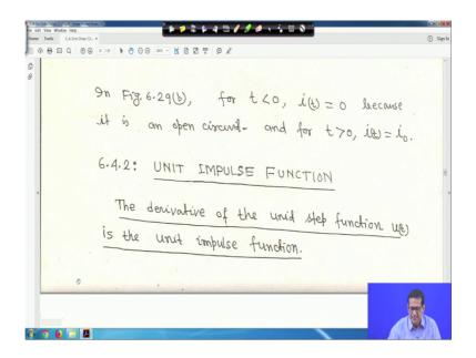
Now, next is that unit impulse function, right. Actually, physically unit impulse function is like ideal sources volt ideal sources or resistor that your unit in physically it is not realizable, but it is a very strong mathematical tool right, for circuit analysis. So, the derivative of the; it is underlined only the derivative of the unit step function u t is the unit impulse function.
