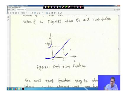
So, figure 32, shows the unit ramp function; that means, for a negative value of t, this is that which is plot like this, it is plotting like this. So, negative value of t it is 0 and for positive value of t it is shown right. And this is unit this is also 1 right. So, this is a unit step, your what you call the ramp function.
