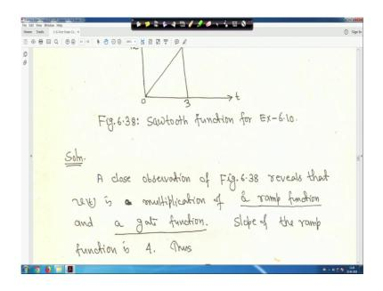
So, a close observation reveals that v t is multiplication of a ramp function, it is a ramp function. And another thing as a gate function and the gate function and this at t is equal to 3. Suppose your what you call, at t is equal to 3 it is your what you call that yours it is going on a ramp and at t is equal to 3 switches off right.
