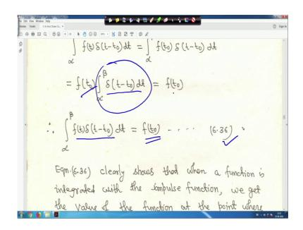
So, here now this is this is come out right. So, alpha to beta delta t minus t 0 d t is equal to f t 0 because this is actually you take that area is equal to your what you call; that unity 1 right. So, that is equal to f t 0, therefore, alpha to beta f t delta t minus t 0 d t is equal to f t 0. So, this is equation 36 right; that means let me move little bit up.
