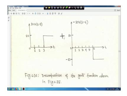
So, now when it is switching on it is a value has given 10 volt, v t right, it is a 10 volt. So, when it is switching on at t is equal to 3, so, this will be actually 10 u t minus 3, right. And when it is switch off switched off at t is equal to 6 second it will be minus 10 u t minus 6, right. So, at the time of switching on it will be 10 u t minus u 3 right, plus and at the time of switching off at t equal to 6 second it will be minus 10 u t minus 6.
