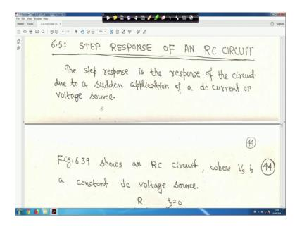
Now, the step response is the response of the circuit due to a sudden application of dc current or voltage source because our interest here is dc transient and that is first order circuit either RC circuit or RL circuit right. So, in this course we will not consider RLC circuit or LC circuit; that is second order circuit we will not consider. And so, the step response is the response of the circuit due to a sudden application of a dccurrent or voltage source.
