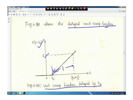
So, it is starting from t 0 and this distance again your this distance is again 1 right, t 0 plus 1 minus t 0 1 this1. So, unit ramp function and this r t minus t 0, this is the plot of the your what you call unit ramp function delayed by t 0; that means, when it is delayed it will be t equal to t 0 on the right on side, that is with the first coordinate right. And when you are that is or starting from here, but this is your this will be less than t 0, it is 0.
