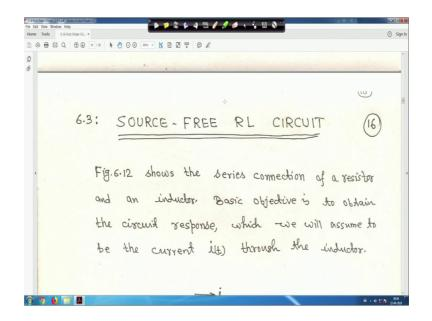
So, philosophy will remain same just as it is inductor, so just we have to see how it happens. So, this figure 12 shows the series connection of a resistor and inductor. Basic objective is to obtain the circuit response which will be natural response, because this is a source free circuit which will assume to be the current it through the inductor.
