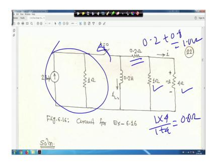
So, in that case what will happen if this is open this 1 ohm and 4 ohm they are in your what you call in parallel right; that means, their equivalent resistance will be 1 into 4 by 1 plus 4 is equal to your 0.8 ohm and with that this 2 ohm resistance is in series. Therefore, 0.2 plus 0.8 equivalent resistance is 1 ohm right and in that case time constant of the circuit will be tau is equal to L by R right.
