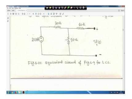
So, this is and this is initial condition that is that is why writing this is 0. So, current through this I told you 20 upon this is open this no current is flowing through 10 ohm resistance, because it is open circuit. So, i is current flowing through this I showed you that this 1 upon 6 ampere then v c 0 will be 90 into 1 upon 6. So, that is why it is 15 volt that is the initial voltage it is 15 volt.
