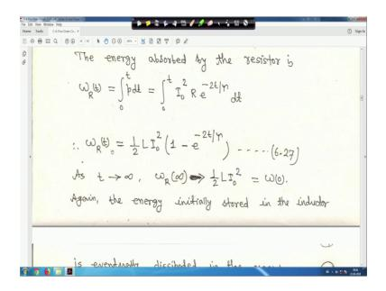
You will get half omega R t is equal to half L I 0 square into 1 minus e to the power minus 2 t upon tau this is equation 27. So, at t tends to infinity that is your omega R infinity is equal to half L I 0 square is equal to omega 0 omega initially also showed. Initially as stored half L I 0 square again the energy initially stored in the inductor is eventually dissipated in the resistor right. So, this is hope these things are understandable to you quite simple quite simple right.
