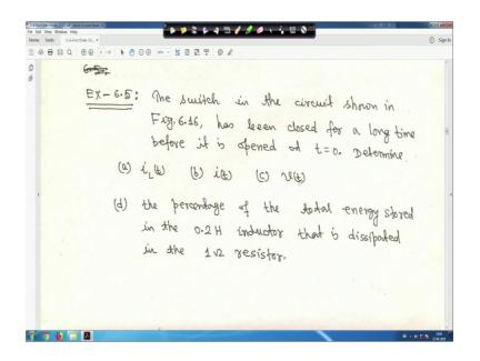
So this is 1 then another one another example is that your the switch in the circuit shown in figure 16, I will show you as been closed for a long time before it is open t is equal to 0. Determine i L t i t and v t that a b c that a is i L t b is it and c this 3 things you have to find out and fourth the d the percentage of the total energy stored in the 0.2 Henry inductor that is dissipated in the 1 ohm resistor right.
