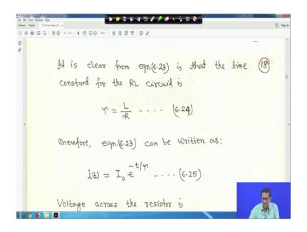
So, this is the plot so this is this is I explain tau is equal to therefore, i t is equal to I 0 e to the power minus t by tau. So, voltage across the resistor is v R t is equal to i into R. So, this is your, I and this is R so substitute I here it will be I 0 into R e to the power minus t upon tau this is equation 25.
