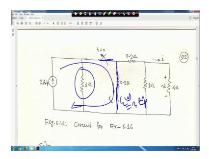
So, this circuit I will show you the switch in the circuit shown in has been closed for a long time before it is open at t is equal to 0 right. So, this is actually this is the circuit
