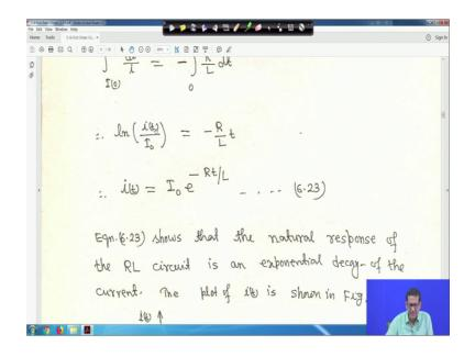
So, now if you integrate it, it will be natural log i t upon small i 0, actually this is small i 0 this is small i 0 and small i 0 is equal to I 0. So, it will be i t upon I 0 is equal to minus R upon L t. That means, i t is equal to I 0 into e to the power minus R t upon L, this is equation 6.23 this is chapter 6. So, this thing now that 23 was natural response of the RL circuit is an is an exponential decay of the current right.
