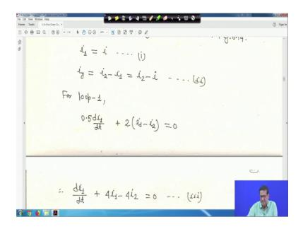
So, it is 0.5 di 1 upon dt then we are moving we are moving here clockwise. So, it will be 2 into plus 2 into i 1 minus i 2 you are moving like this because i 1 is going upward and i 2 moving downwards. So, resultant upward is i 1 minus i 2, so plus 2 into i 1 minus i 2 is equal to 0 or you just multiply both side by 2, then you will get di 1 by dt plus 4 i 1 minus 4 i 2 is equal to 0 this is the equation 3 given.
