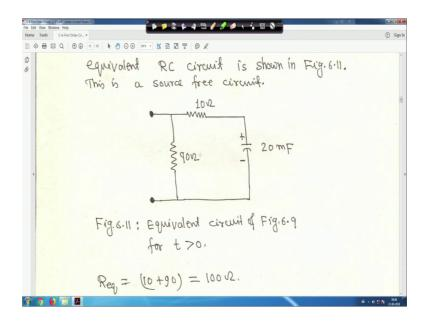
So, in this case your this is the equivalent circuit right, this is the x 10 ohm and 90 ohm are in series that it is 20 millifarad and initial capacitor was charged at v c 0 is equal to 15 volts that you have seen right. So, if then 40 then your R eq equivalent will be 10 plus 90 so 100 ohm.
