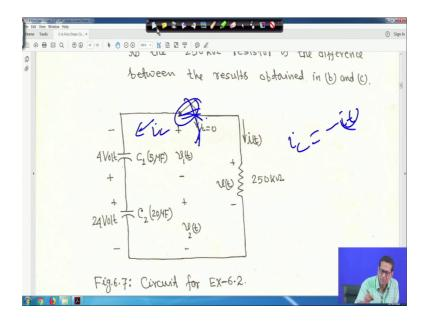
So, this is the i t and say this is current is flowing i c. So, here also i C is equal to i C is equal to then minus it because i C plus i t is equal to 0, this is closed apply case some point at KCL right. So, i C is equal to minus i t right so; that means, i C is equal to one is
