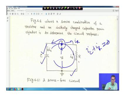
So; that means, figure 1 suppose it shows us series combination of a resistor and an initial energy your charge initial sorry initially charged capacitor. So, main objective is to examine the circuit response.
