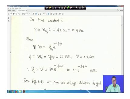
And v is equal to you know V 0 e to the power minus t by tau, but V 0 is given 10 volt. So, V 0 is equal to V 0 is equal to v c 0 is equal to 10 volt it is given and tau is equal to 0.4 second therefore, v c is equal to v is equal to 10 e to the power minus t upon 0.4. So, that is 10 e to the power minus 2.5 t volt, this is the simple thing from the previously developed your formulas we are just putting the data.
