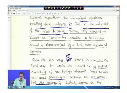
So, the differential equations resulting from analyzing R C and R L circuit, that is your the differential equation resulting analyzing that R C and R L circuits are of the first order right hence it is underlined the circuits are known as first order circuits. A first order circuit is characterized by first order differential equation. So, there are two ways it will be 2 right, I am correcting it right.
