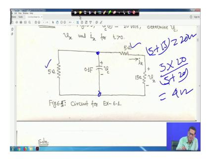
So, here your a simple circuit of a this thing is taken, a series parallel your parallel circuit right. So, 5 ohm resistor is there, 0.1 microfarad capacitor sorry 0.1 farad is there, voltage across is v c this 5 ohm resistor and this is 55 and 15 both are in series and taken separate given separately and current through is i x. And voltage across 15 ohm resistor is vx you have to you have to find out initial values of the your capacitor voltage that is
