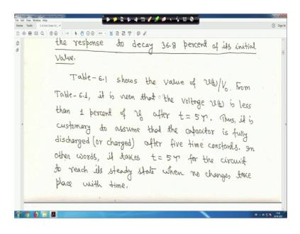
So, that means equation 13 we can state that the time constant of a circuit is the time required for the response to decay, 36.8 percent of its initial value. This is 0.368; that means, if you take in percentage that is 36.8 percent of initial value is V 0 right.
