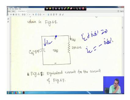
Same we are drawing this is vt this is the equivalent circuit of that one right. Now the time constant is tau is equal to RCq 250 into 10 to the power 3 it is kilo ohm. So, converted into ohm into 4 into 10 to the power minus 6, 4 micro farad so, that is 1 second
