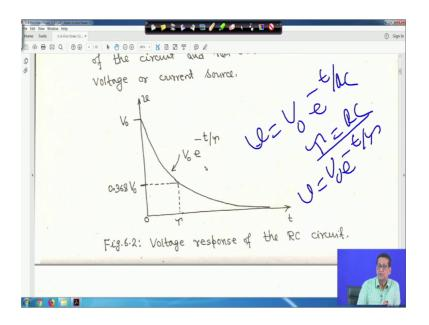
So, now if we plot if we plot that V is equal to V 0 e to the power minus t upon tau, that is your that is v v is equal to your V 0 e to the power minus t upon R C, if we take tau is equal to R C then v is equal to V 0 e to the power minus t upon tau, tau is equal to R C tau actually is called the your time constant right will see that.
