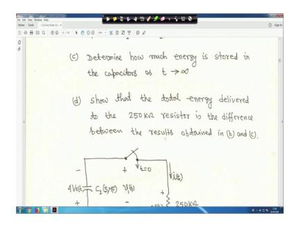
Next is determine how much energy stored in the capacitor and t tends to infinity and so that the stored energy delivered to that 250 kilo resistor is the difference between the result obtained in b and c. So, these are the 4 thing you have to make it right.
