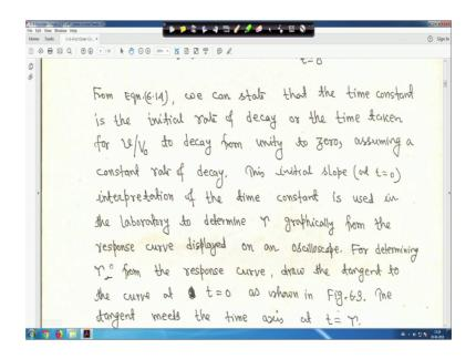
So, for determining tau from the response curve, draw the tangent to the curve at t is equal to 0; that tangent meets the time axis at t is equal to tau; that means, that t is equal to 0 at t is equal to 0 if you draw a tangent it will meet here at tau right here it will meet at tau right.
