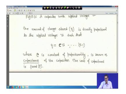
So, the amount of stored amount of charge q is directly proportional to the applied voltage v such that q is equal to c v this is you know also from your physics right, so as similarly physics. So, as c is constant of proportionality is known as capacitance of the capacitor right. And the unit of the capacitance is farad right. So, this you know that q is equal to c v.
