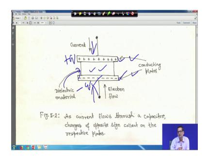
So, it is this is this is shown the direction of the current that current flows; and electron it is given that flowing upward actually and in between this is your dielectric material. And these two this one and this one these two are conducting plates. So, as we have taken the direction of the current moving upward. Generally in any metals right that you are what you call that whenever current flows means it is basically your what you call that moving of your electrons right.
