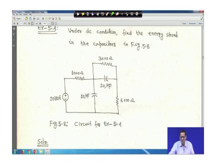
So, now under dc condition now find the energy stored in the capacitor in figure 5.8.So, this is my figure 5.8. We will have to find out that what your the energy stored in the capacitor. So, this is 1000 ohm, 3000 ohm, 6000 ohm, and this is 20 micro farad, this is 10 micro farad. Now, we will we will redraw the circuit right under dc condition that that 10 micro farad 20 micro farad it will be open at steady state right; and 20 volt dc is applied. So, if you read out the circuit, this is open.
