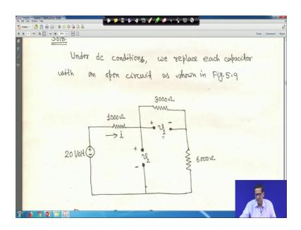
Say voltage across this 20 micro farad is b 1, this voltage is b 1, and this voltage is b 2 right. So, this is open. So, this is open. So, this current is i, this i is flowing like this; i is flowing like this right because this is open this is open right. So, 1000, 3000 and 6000, so 10,000 ohm right.
