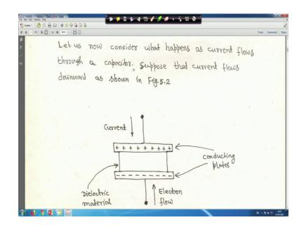
Ok, so let us come to this topic capacitors and inductor. We have just started with that right. So, now you know let us consider what happens as current flows through a capacitor right. Suppose that current flows downwards as shown in this figure, in this figure right.
