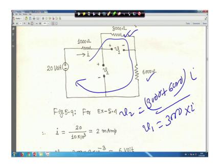
This same current i is flowing through this right. So, b 2 will be actually b 2 will be this 3000 and 6000, 3000 plus 6000 into i that will be your b 2 because this 3000, 6000 are in series right. And b 1, b 1 will be 3000 into your i because this is the voltage across b 1 is the voltage across the 3000 ohm resistance. Once you get this b 1 and b 2, you know c 1 and c 2 you can calculate half c v 1 square and half cv 2 square the energy stored right.
