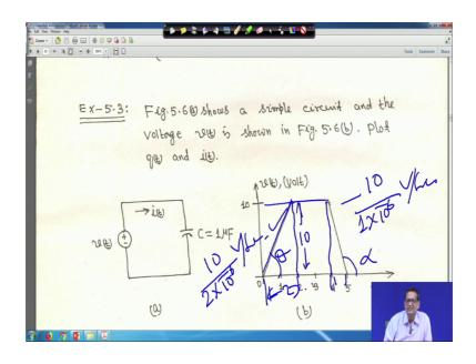
So, this easy example easy example, now, next one is figure 5.6 say that is I will say 6.a because that it is chapter five. So, is a simple circuit? And the voltage v t shown in figure 5 this 6 b. You have to plot q t and i t. Now, question is it is given your this circuit is given. This simple series circuit and one voltage source is connected with the capacitors
