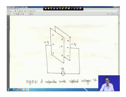
Suppose a voltage is applied between the two your two plate the two plates, so this side this is the plus terminal of the voltage right source and that is why plus charge is accumulated and minus q will be accumulated and total charge will be 0 right. So, when you says to capacitors total charge if the either of the plate, it is plus and this is minus. So, this is simple diagram. (Refer Slide Time: 05:29)
