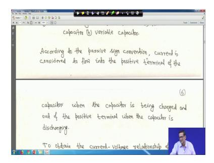
So, just now I told you according to passive sign convention, current is considered to be flow into positive terminal of the capacitor, when the capacitor is being charged right. And your and out of the positive terminal I told you, when the capacitor is discharging. (Refer Slide Time: 08:02)
