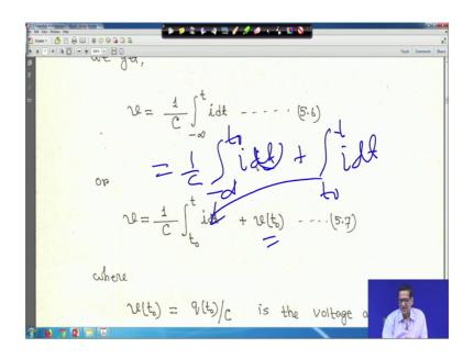
Actually this equation this equation this equation if I write like this, 1 upon c sometime say minus infinity to t 0 right. If we write i dt right, so if we right i dt then plus then t 0 to t then i dt this way you can write. So, this equation is here, this is this equation right t 0 to n. So, this equation 1 by c you are writing actually your what you call that is v t 0 here what you call v t 0 this equation you are writing actually. This let me clear it.
