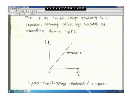
This is the current and voltage relationship for a capacitor, assuming positive sign convention the relationships shown in figure 5. This side is i. This side is dv by dt the rate of change of voltage; this is i and this is the slope c right. So, it is a linear it is it is a linear equation basically right. Therefore, c when c is independent of i your db by d.
