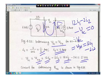
It is basically 12 i 1 minus 2 i 2 then encountering minus terminal first. So, minus V oc, V oc is V Thevenin is equal to 0 that means, V oc say you write is equal to V Thevenin is equal to 12 i 1 minus 2 i 2, that is what I have written V oc is equal to V Thevenin is equal to 12 i 1 minus 2 i 2 that is 12 into 3 minus 2 sorry 1 by 3 minus that is 2 into 1 is equal to 2 volt. So, V Thevenin is equal to 2 volt right.
