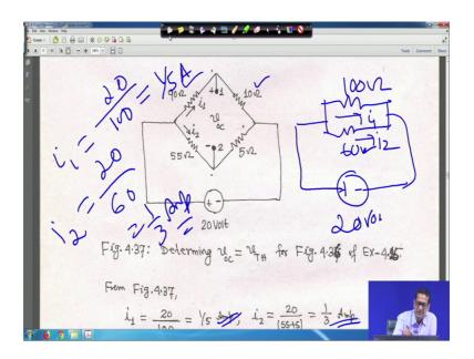
So, basically it is 100 ohm right and similarly 55 and 5 ohm both are in series. So, it will be your 60 ohm and with that this 20 volt plus minus is connected, this is 20 volt right and current through this it is i 1 and current through this it is i 2 right. Therefore, i 1 is equal to your 20 volt divided by 100. So, it will your become 1 by 5 ampere right, that is here it is i 1 is equal to 1 by 5 ampere.
