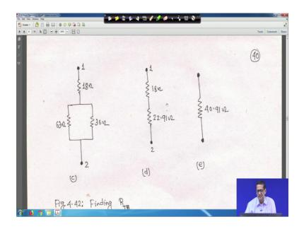
So, if you let me clear it that is what we have made it that 18 ohm and 63 and this parallel if this two are in parallel. So, equivalent towards coming 22.91 and ohm and 18 18 ohm is in series. So, total is 40.91 ohm. Now R Thevenin is 40.91 and here, it is your here it is 40.91 and V Thevenin in that with that you connect, now the 50 ohm resistance which was taken off right. So, you will get the current and that is the current flowing to 50 ohm resistance. So, let me clear it.
