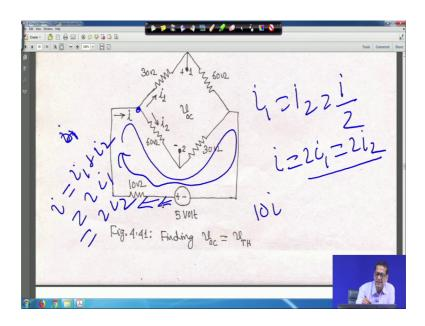
That means i 1 actually is equal to i 2 is equal to i by 2, because whatever current is entering at this point, it will half of the current of half of I will go here half of I will go here. So, i 1 is equal to i 2 is equal to i that means, i is equal to 2 i 1 right is equal to 2 i 2.
