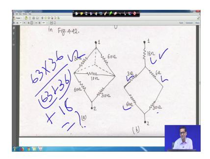
And with that this combine is in parallel that means, it is equivalent is 63 your this is 63 ohm and this is 36 right, divided by 63 plus 36 whatever it comes with that 18 ohm is in series with that so, that is equal to what right.
