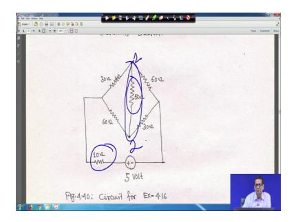
Previous case there was no there was no resistor here, but one 50 ohm 10 ohm resistance is there and you have to find out that what is the current through the 50 ohm resistance say this terminal you mark at 1 and this terminal you mark at 2 right and then, you follow and so, first is we have to open this resistance 50 ohm resistance.
