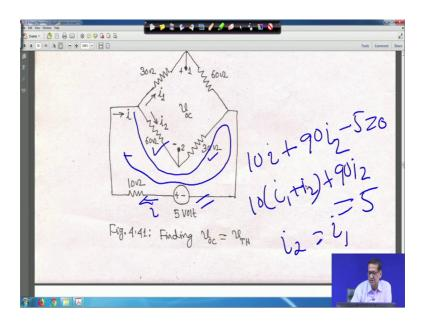
So, i is flowing through this is i so, 10 into i right plus we are move we are moving like this; we are moving like this we are moving like this plus your this i 2 current is flowing through 60 and 30; So, 90 i2 90 i2 right, then minus 4 is equal to 0 because this 5 volt so, right but i were, but question is that 10 i is equal to i 1 plus i 2 plus 90 i 2 is equal to 5 right, but i 2 is equal to i 1. If you put it here, then you will get i 1 solution for i 1 and i 2.
