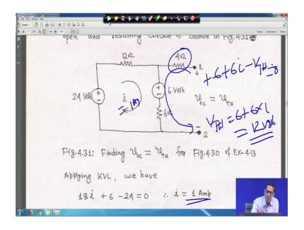
So, I can write here plus 6 right and i is equal to you got 1 ampere right; so, plus 6 plus 6 into i minus V Thevenin is equal to 0 because it is encountering negative terminal passed. Therefore, V Thevenin is equal to 6 plus 6 and i is equal to 1 so, that is your 12 12 volt. So, V Thevenin is equal to 12 volt here, it is already solved here everything is solved here.
