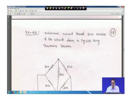
So, next is you determine the current through 50 ohm resistor of the circuit, shown in figure 40 using Thevenin's theorem, in this case difference between the previous one and
