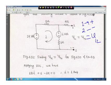
So, first let me clear it so that means, this one if you come that you have to find out your V your, what you call the V Thevenin is equal to; so, R L is equal to 4 ohm is opened here right, and your basically this one is equal to V 1 2, when we write 1 2 1 terminal means it is plus and two means it is minus right. So, V o V Thevenin V oc that V open circuit voltage is equal to V Thevenin actually is equal to V 1 2 right.
