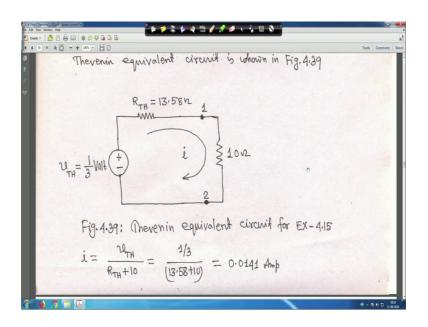
And with this this 10 ohm your this 10 ohm now is connected here, 10 ohm is this is your V Thevenin one-third volt R Thevenin is this one and 10 ohm is connected here with that. So, ultimately you will get V Thevenin by R Thevenin plus 10 right is equal to one-third 13.58 plus 10. So, this is actually 0.014 ampere this is your i right so, this is easy to understand.
