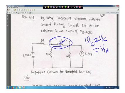
Next one is by using Thevenin's theorem determine current flowing through three ohm resistor between 0.1 and 2 right. So, this is the problem that you have to find out the
