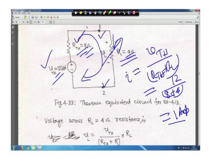
So, next is this that means, this is your V Thevenin, this is your V Thevenin with that R Thevenin is there in series 8 ohm. And now you connect that R L is equal to 4 ohm resistance in terminal work loss terminal 1 and 2. So, if you do so, then current flowing through this you find out; so, total resistance here it is 8 ohm, here it is 4 ohm 12 ohm. Therefore, i is equal to say V Thevenin by R Thevenin plus R L right.
