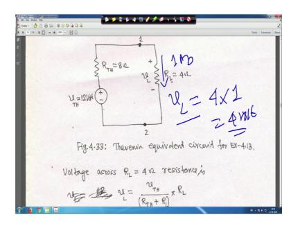
So, let me clear it. Therefore, your V l is equal to your 4 and current flowing through this is 1 ampere. So, it is 4 into 1 that is your 4 volt right. So, voltage across this load resistance is equal to 4 volt. So, let me clear it; So, that is that is why this is we have got that 4 volt right, here it is here it is 4 volt right V L is equal to so, next one varieties of problem we have taken.
