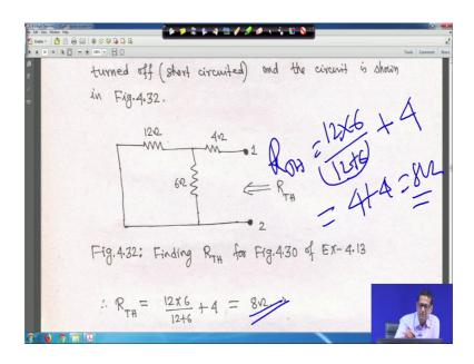
So, for R Thevenin that voltage source is short circuited right. So, if voltage source is short circuited for R Thevenin; that means, here this source is short circuited, this is short circuited and this is short circuited that means, this 12 ohm is and 6 ohm are in parallel with that this 4 ohm is in series that will be your R Thevenin.
