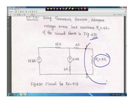
So, using Thevenin's theorem, you determine voltage across low resistance R L of the circuit shown in figure 30 right. So, this is your its chapter 4.30 you are making. So, it is a figure 30 right. So, we have to find out using Thevenin's theorem that your current through load resistance R L is equal to 4 ohm. So, for Thevenin's theorem, what we will do? First we will remove this load resistance right, we will make an open circuit right that what you have done right.
