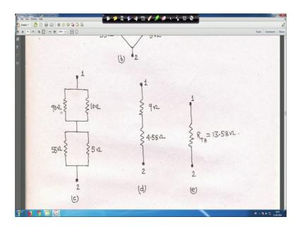
After that these two are shown 90 and 10 and 55 and 5 are in parallel, then this is 9 ohm and equivalent to this it is coming 4.58. So, total is R Thevenin is equal to 13.58 ohm right.
