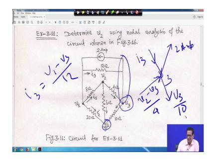
So, this 2 ampere current is you are leaving this node right there another thing is that that i 3 current this is that i 3 is marked here. So, this i 3 current actually entering into the node and i 3 I told you earlier that i 3 is equal to v 1 minus v 3 v 1 minus v 3 by 12 these 2 currents are entering right.
