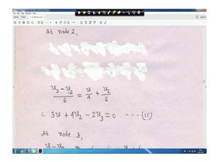
Similarly at node 2 here directly I am writing at node 2 that v 3 minus v 2 upon 6 is equal to v by 4 that is v 2 upon 6; that means, at node 2 this is actually this is actually node 2 right, this
