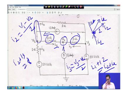
So, this i 1 current entering into the node so, this current is i 1 this is entering into the node, then i 2 current emitting like this the way we explain that KCL this is your i 2 current it is leaving the node then this is a common node then 12 ampere current it is entering into the node because direction is this way entering into the node. So, this is 12 ampere current right.
