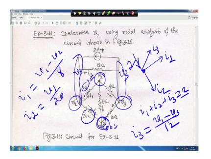
Next one is determine v 2 using node analysis of the circuit shown in figure this thing right here also directly I write those equations, but this is a bridge circuit right. So, here this is your reference node and you have this is node 1, this is voltage v 1, this is voltage v 2 and this is voltage v 3 right and 1 2 ampere source is connected basically this this is a common node right.
