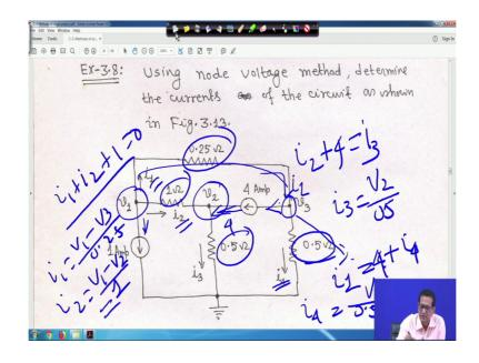
So, if this circuit is given right you have to find out the currents of these whatever is given right. So, you are using the node voltage method, you have been asked to find out the current.
