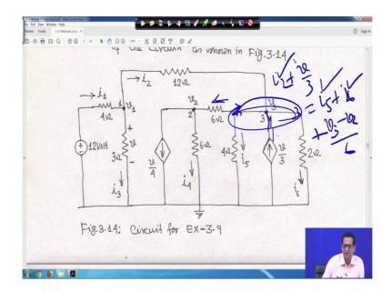
So, basically this is a common node this is a common node right this is 3 this is whatever it is this is a common node. So, in this i 2 current is entering this current i 2 is equal to v 1 minus v 3 by 12 this current is entering.
