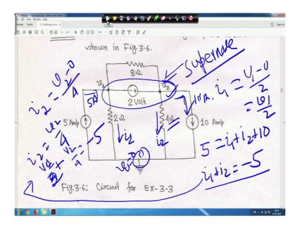
This is actually super node this is supernode because 2 1 voltage source is there in between 2 non reference node; so, in this case, a 5 ampere current this 5 ampere current actually entering the super node. And this 10 ampere current actually it is leaving the supernode and this is node 1, say this is also current leaving the supernode, say i 1 and this is the currents at node 2, this is the i 2, right.
