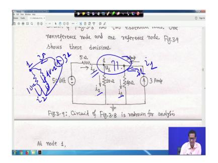
So, just for the purpose of this thing, this circuit is redrawn and voltage actually, this I told you this is actually a single node. So, basically this one because no electrical element is here no electrical element is so, basically it say node 1, right only v 1 and this side is plus minus 50 volt and this is your i 1, this current, we have taken i 2 and this current is i 3 and this is 3 ampere.
