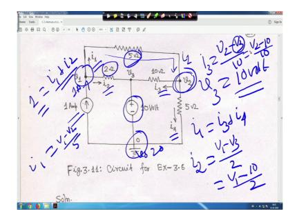
Look, in this case, in this case, you have one current source here for 1 ampere; that means, this current actually this current is 1 ampere this current is 1 ampere entering into the node, right and next if voltage source is there here 10 volt and this is your node 3 and this is your reference node. So, here voltage v 0 is 0, yes, again and again I told you; so, basically directly actually v 3 is equal to 10 volt, right; so, this actually 10 volt right.
