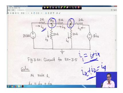
And similarly at node 2 if you apply KCL, then your because this current is incoming and these 2 are outgoing at and at node 2 your i 2; i 2 and i x entering into the node 2 and this i 4 is leaving. So, it is i x plus i 2 is equal to i 4 these 2 equations you have to write to after that you put in terms of v 1 and v 2.
