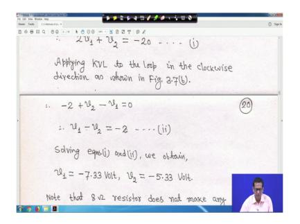
So, let me clear it. So, this is your v 1 minus v 2 is equal to minus 2 or v 2 minus v 1 is equal to 2, right. So, solve this 2 equation that equation 1 and equation 2, you solve it, then you will get that v 1 is equal to minus 7.33 volt and v 2 is equal to minus 5.33 volt note that 8; 8 ohm resistor; that means, this one you note that 8 ohm resistor does not make any difference because it is connected across the supernode.
