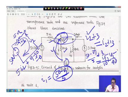
Then it will be i 1, this current is entering at node 1, this is 3 ampere current, I mean this is the same thing this is same thing this 3 ampere current, I told you that all are connected at same point, then i 1 plus 3, these 2 are your this current are entering into the node 1 and i 2 and i 3 leaving.
