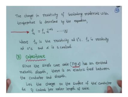
Therefore, the change in resistivity of insulating materials with temperature is described by the equation these rho t is equal to rho 0 e to the power minus alpha t, this is equation 4. Now, where rho t is the resistivity at t degree Celsius, rho 0 is resistivity at 0 degree Celsius and alpha is a constant.
