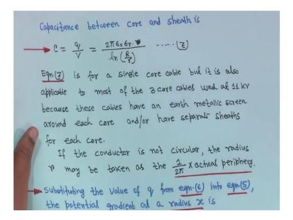
Therefore capacitance will be between core and sheath is your c is equal to q by V if you substitute it will be q by V will be 2 pi epsilon divided by 1 n capital R by small r, this is equation 7. Next, is that equation 7 is for single core cable, but it is also applicable to most of the 3-core cables. This is the 3-core cable used at 11 kV because these cables have an earth metallic screen around each core and or have separate sheath for each core.
