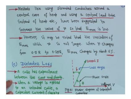
So, method like using stranded conductors around a central core of hemp and using a central lead tube instead of hemp etcetera have been suggested to increase the value of r, so that, E max is low. However, it may be noted that the variation of E max with r is not large, when r changes from 0.5 R to 0.25 R, E max changes just by about 6 percent. But, some ideas you have regarding this E max, minimum value of E max.
