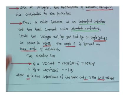
So, thus a cable behaves as an imperfect capacitor and the total current under unloaded conditions, leads the voltage not by ninety degree, but by an angle 90 degree minus delta; that means, it has some what you call it is not a pure capacitance, but it has some imperfect capacitor we call, because losses occurs that dielectric absorption also contribute to the power loss.
