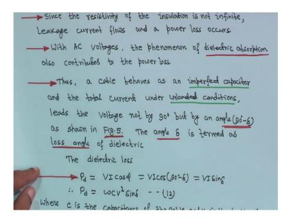
So, in that case what will happen, since the resistivity of the insulation is not infinite, leakage current flows and a power loss occurs because insulation resistivity is not infinity. So, leakage
