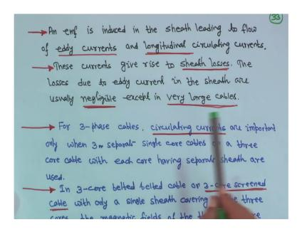
An EMF is induced in the sheath leading to flow of eddy currents and longitudinal circulating currents, but this current give rise to the sheath losses. So, there will be some power loss in the sheath. The losses due to eddy current in the sheath are usually negligible except in very large cables. Very large cable means high voltage cables, at the same time, long, very long cables in terms of kilo meters. So, otherwise that eddy current loss is negligible.
