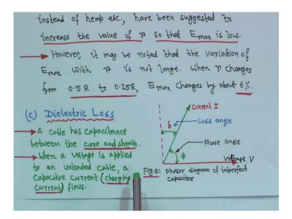
Next, we will come to the dielectric loss; this is another important aspect for the cables. So, this diagram I will come later. So, a cable has capacitance between the core and the sheath that we have seen when a voltage is applied to an unloaded cable, a capacitive current that is charging current flows.
