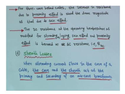
Now for three-core belted cables, the increase resistance due to proximity effect is about the same magnitude as that due to skin effect. I mean, both increase will be affected same for proximity and your skin effect. The DC resistance at the operating temperature as modified for stranding, laying, then skin effect and proximity effect is termed as AC resistance, that is, R ac. We refer as a R ac.
