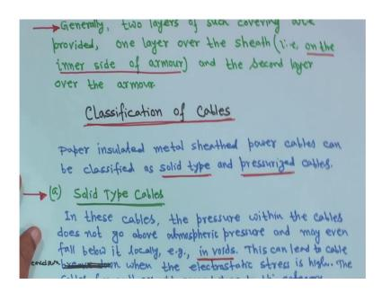
But, next is the generally, 2 layers of such coverings are provided, one layer over the sheath and there on the inner side of armour and the second layer over the armour. Now, before classification to your these thing cable, first I will show you one diagram and then this thing.
