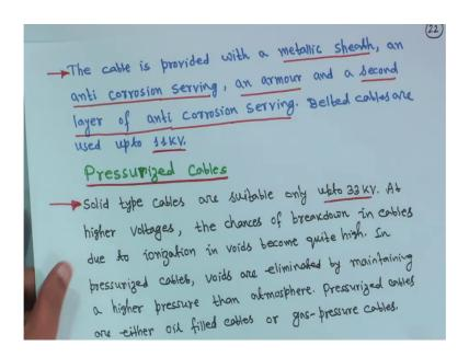
So, the cable is provided with metallic sheath, an anti corrosion serving, an armour and a second layer of anti corrosion serving. Belted cables are used up to 11KV.
