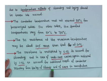
The resistance is multiplied by 1.02, that means 2 percent increase, to account for stranding and in case of multi core cable again multiplied by 1.02, that mean 2 percent increase, to account for additional length of conductor resulting from the lay of strands and of core in manufacture. So, these 2 percent your things you have to multiply, so that more or less you will get that your what you called that more or less accurate values.
