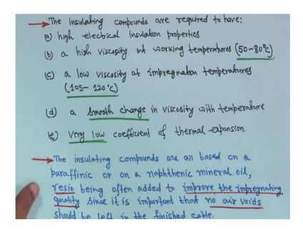
The insulating compounds are required to have; high elect insulation properties, then high viscosity at working temperatures see 50 to 80 degree Celsius normal, in low viscosity at impregnation temperatures that is 105 to 120 degree Celsius, a smooth change in viscosity with temperature and very low coefficient of thermal expansion. So, these are the insulating compounds are required to have particularly the very low coefficient of thermal expansion.
