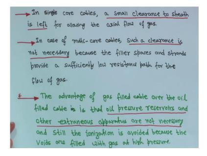
And, if void formation is just hold on, there in single core cable is a small clearance to sheath is left for allowing the axial flow of gas. So, there should be a small clearance to sheath is left for allowing the axial flow of the gas. In case of multi core cables, such clearance is not necessary because the filler spaces and strand provide a sufficiently low resistance path for the flow of gas.
