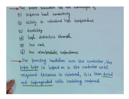
So, the paper insulation has the advantages of superior heat conductivity, then ability to withstand high temperature, then durability, then high dielectric strength, low cost and low electrostatic capacitance. So, these are the your advantages for paper insulation and for providing insulation over the conductor the paper tape is lapped on to the conductor until required thickness is obtained. So, it is then dried and impregnated with insulating compound.
