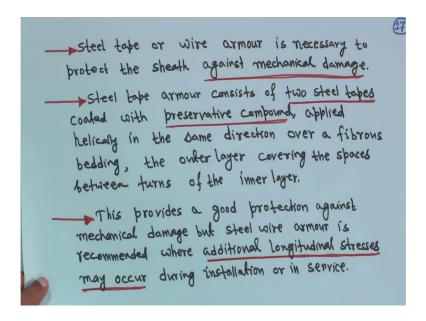
So, steel tape or wire armour is necessary to protect the sheath against mechanical damage look. We are protecting insulation for the sheath now steel tape or wire armour is necessary to protect the sheath against mechanical damage; that means, another round you have to use for steel tape or wire one after another. So steel tape it is like your onion know, one after another.
