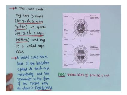
Next is that in this is belted cables three-core and 4 core I will come to that. So, the multi core cable may have three-cores that is for 3-phase 3 wire system or 4 core that is 3-phase 4 wire systems and may be a belted type cable. So, a belted cable has a part of the insulation applied to each core individually and the remainder in the form of an overall belt as shown in figure-2, a and b.
