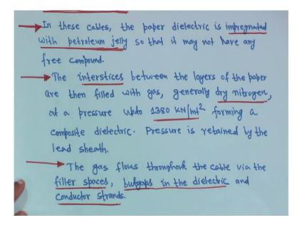
Next, one is that your what you call that gas filled cables. So, in this cable the paper dielectric is impregnated with petroleum jelly so that it may not have any free compound. The interstices between the layers at the paper are then filled with gas, generally dry nitrogen at a pressure up to 1380 kilo Newton per meter square forming a composite dielectric. Pressure is retained by the lead sheath. So, this is for gas filled cables.
