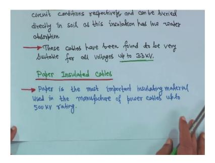
So, diagram and other thing cables I will come to that I will show you from the book only, but later. So, paper is most important insulating material used in the manufacture of power cables up to 500 KV rating. So, this paper insulated cables are very common.
