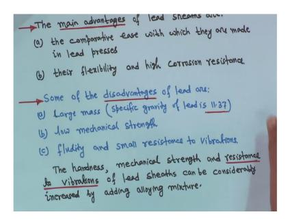
So, the main advantage of lead sheath, the comparative ease with which they are made in lead presses; second, their flexibility and high corrosion resistance. These are the advantages. The disadvantages; large mass because specific gravity of lead is 11.37, low mechanical strength and fluidity and small resistance to vibration; these are the disadvantages of lead.
