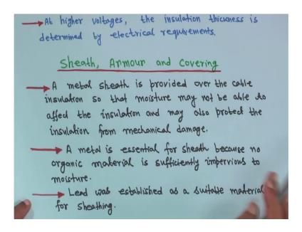
Next, one is diagram I will come later. Next, is sheath armour and covering. So, generally a metal sheath is provided over the cable insulation so that moisture may not be able to affect the insulation and may also protect the insulation for mechanical damage; that is why a metal sheath is provided over the cable insulation.
