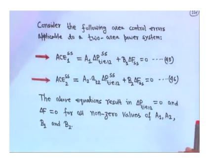
Now, question is consider the following area control errors applicable for a two-area power system. Suppose, ACE we know ACE is equal to we know that we have seen that is your B 1 ACE 1 is equal to B 1 delta F delta F 1 plus delta P tie 1 2. Now, what you can do is suppose ACE 1 steady stable multiplied by some constant A 1 capital A 1 into
