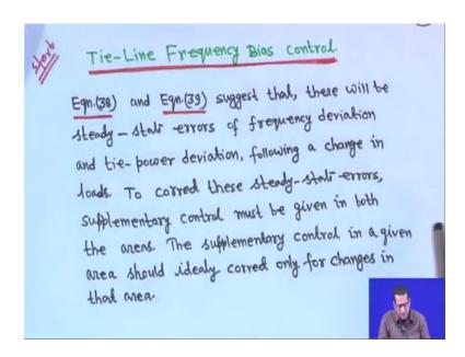
Now, another next is the tie line frequency bias control, right. So, that means, these two equations 38 and 39, it suggest that if your system will uncontrolled then there will be an error in your steady state error of frequency deviation as well as you tie power deviation following a load disturbance, right.
