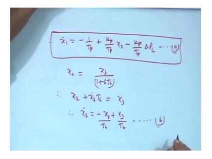
Similarly, when we will come to x 2, x 2 is equal to X 3 into 1 upon 1 plus STt. So, x 2 is equal to x 3 upon 1 plus ST t cross multiply. Therefore, x 2 S x 2 means - x 2 dot TT is equal to x 3. That means x 2 dot is equal to minus x 2 plus 3. Divide! This is, your what you call - divided by TT divided by TT. So, this is equation, your what you call say - equation B. That means, for this equation, this equation x 2 dot is equal to.
