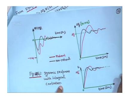
I will show you some pattern of response. If you plot this, so, there will be no steady state error. This is the frequency deviation. So, at it will after some transient oscillation, it will settled to your deviation, will settled to 0. So, black one is non - reheat and for reheat type, it is slightly peak; is slightly higher and slower because of the reheat time constant is there.
