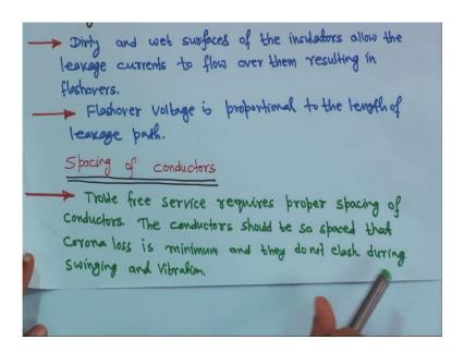
Next one, is that spacing of conductors; you have seen for transmission line 33 kV, 66 kV, 132 kV or 220 kV or above you have seen different type of conductor spacing are there, also in each space you can see 2 conductors or 4 conductors are there in each space. Recently, I went somewhere, I found that 4 conductors are there in each space and you know why we use that 2 conductors or 4 conductors or even more for high tension transmission line that if I use that; so spacing of conductors.
