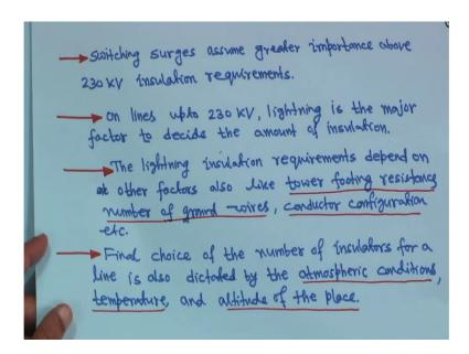
Next, is that your switching surges assume greater importance above 230 kV insulation requirements; in our country 220 kV or above 220 when 400 kV line, so, 230 kV installation requirements. Now, on the lines up to 230 kV lightning is the major factor to decide the amount of insulation, because lightning stroke is very common phenomena in our country, everywhere all over the world and you have to protect all these things on the lightning is the major factor to decide the amount of insulation.
