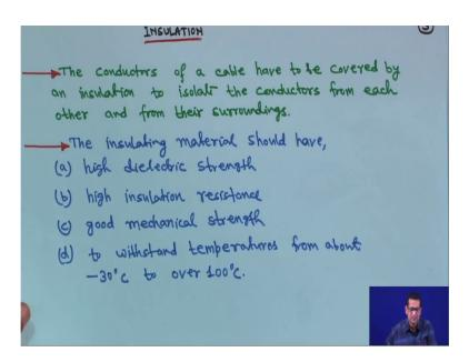
Therefore, when we come to the insulation the conductors of a cable have to be covered by an insulation to isolate the conductors from each other and from their surroundings; suppose, if you have a 3 phase line and 3 core cables then each 1 has to be insulated from each other, otherwise there will be short circuit. Therefore, insulation is more important.
