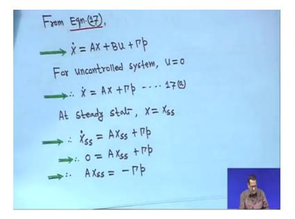
So, next is that that is one thing and now next is that X dot is equal to AX plus B u plus gamma p. We have seen this 10 have to call this state space analysis this stay all these equations we have seen A B gamma, right? And X A is as told you state transition matrix B is the control transition matrix and gamma is the disturbance transition matrix.
