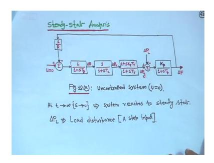
So now look steady state analysis, first part we will see the steady state analysis that suppose this is your control signal u is 0 uncontrol mode when u is 0 uncontrol mode and this is your this part is governor then turbine then generator, right? So, and as usual we will see what is the steady state value of delta f delta Pg here delta Pv delta E is not our interest, but we will see all these things and uncontrolled mode when there is no controller so u is equal to 0.
