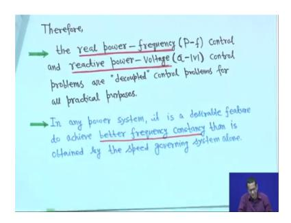
So, that is why the real power frequency we call P-f control right and the reactive power voltage we call q v control it is magnitude written here right problems and decoupled control problems for the all practical purposes right.
