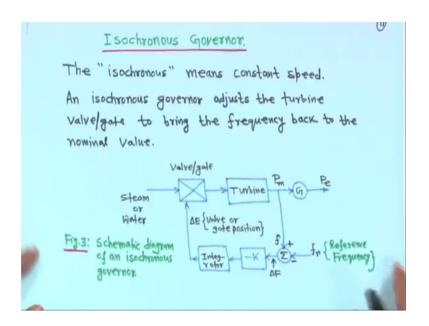
Isochronous governor means that it is a constant field your what you call isochronous meaning is the constant speed. So, an isochronous governor adjust the turbine valve or gate to bring the frequency back to the nominal value right if; that means, it will try to bring your what you call it will adjust the I mean it control actually, in the case of steam
