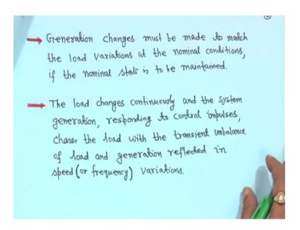
So, question is that generation changes must be made to match the load variation; that means, suppose, when there is a change in load, suppose, there is a increase of load. So, generation actually power system actually chases the load right sometimes, we call it is a load following generator chasing the load or following the load. So, it is a load following.
