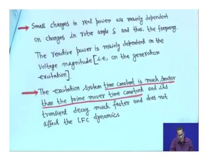
Now, small changes is real power are mainly dependent on changes in rotor angle delta right this is very simple and that is the frequency, the reactive power is mainly dependent on the voltage magnitude that is called the generation excitation that is this side, right that is the this side excitation side right.
