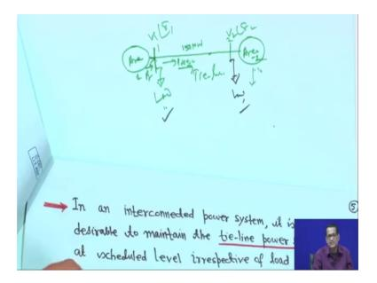
Suppose, we have one power system here, what is area 1 and area 2, later will comes suppose, this is one power system, it is collected by the 3 phase tie line of course, this is your area 2 right and this is your this is actually tie line this is 3 phase line actually tie line means these two powers are interconnected and tied together that is why you call tie line.
