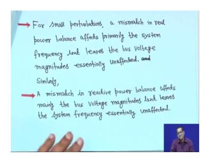
So, for small perturbation when I mean disturbance is very small right a mismatch in the real power balance affects primarily the system primarily the system frequency same concept that decoupled load flow, I have use know. So, almost same thing; but leaves the bus voltage magnitudes essentially unaffected.
