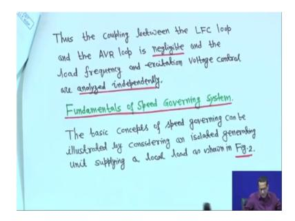
There is the coupling between the LFC loop and the AVR loop is negligible better, you avoid this and the load frequency and excitation voltage control are analyzed independently they are separate right they are separate.
