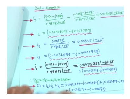
So, second iteration this small i 2 will be 0.004; this is the load P 1 2 minus j Q 1 2 upon that V 2 conjugate right. So, it is V 2 is equal to 0.98773 angle minus 0.62; its conjugate will be this angle will be plus right. So, it will be 0.98773 angle 0.62 degree. If you simplify if you just simplify then i 2 will become 0.005062 an angle minus 37.49 degree. So, if you just is equal to it is i 2 is equal to 0.004 01649 minus j 0.0030809.
