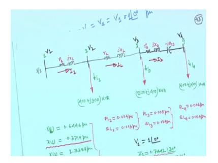
Now, with for the same example just for the purpose of your understanding, what I will do for the same example I have taken a series capacitor also and in the case of series with the same example I have written r 1, x1, r 2, x 2, r 3, x 3 just to show that series capacitors somewhere in distribution line connected, but same Z 1, Z 2, Z 3 value will be used identical thing. Throughout this thing just to have a feeling same parameters are
