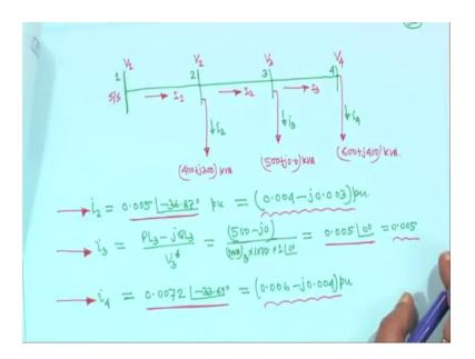
Therefore, it is 500 plus j 0 because this one is totally compensated by this one right. So, in that in that case your and work for this one what we will do? We will use only the first method of the load flow. Second method I have not done it here, but I request you can check also using the second method.
