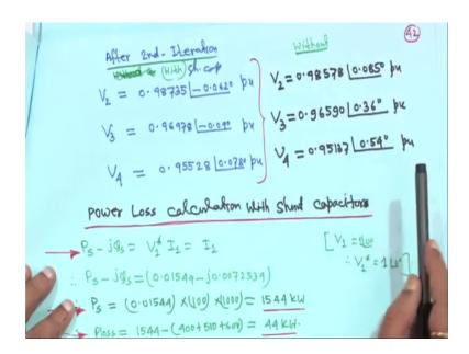
This is after second iteration this is with shunt capacitor right this is with shunt capacitor. So, after second iteration V 2 is 0.98735, here it is 0.98578. So, there is a slight improvement I mean because this is a small system. So, voltage improvement is here because it is 578; it is 735 right.
