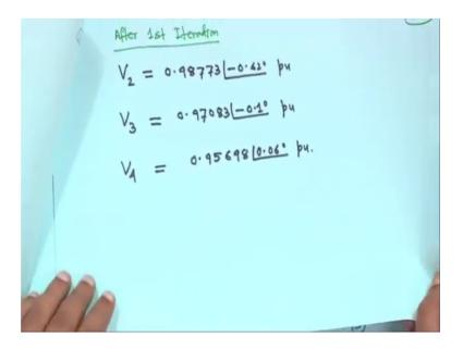
So, after first iteration these are the voltages; V 2 is given whatever we have got it V 3 is given and V 4 is given. This two are lagging angle; although angle is very small and negligible, but and this one is leading angle.
