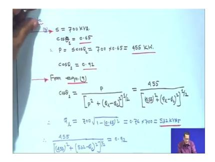
So, in that case S given 700 KVA, it is 700 KVA. Initial power factor is given cos theta 1, 0.65. So, P is equal to your apparent power into cos theta 1. So, a cos theta 1 is equal to 700 in to 0.65 is equal to 455 kilowatt right. So, cos theta 2 is equal to say input power factor is 0.92 from equation 9 we will get cos theta 2 is equal to P upon root over P square plus Q I minus Q c whole square it is putting a half root over.
