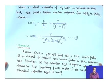
So, assume that a 700 KVA load has a 65 percent power factor is cos pi cos theta is equal to 0.65 it is desired to improve the power factor 2.9 to that is 92 percent means 0.92 determine the following the capacitor size required. What would be the resulting power factor if the next higher standard capacitor size is used?
