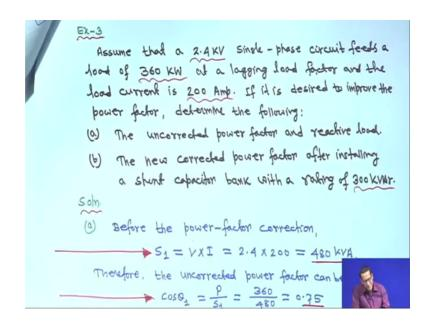
Now, example 3 assume that a 2.4 kilo volt single phase circuit feeds a load of 360 kilowatt and lagging power and at a lagging load power factor and the load current is 200 ampere right if it is desired to improve the power factor determine the following right.
