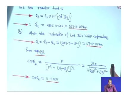
So, now and the reactive load is that S 1 is equal to that cos theta 1 is 0.75. So, theta 1 is cos inverse theta 1. So, you can calculate easily at instead of calculating directly I am writing S 1 into sin of cos inverse theta 1 right. So, Q 1 is equal to S 1 is 480 and this part will be 0.661 that is 317.5 kilowatt that is your reactive load demanded at the your load right.
