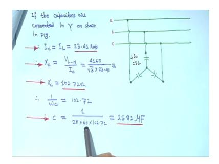
So, now if it is a star connected then I L is equal to I C, if it is star connected one I am showing in every phase that I L is equal to I C, I forgot to mention it here that is why I write here I L is equal to I C it is a star connected right. So, in that case if the capacitors are star connected then I C is equal to I L is equal to 23.41 ampere right. In that case your you have to take the line to new line to line voltage because it is a star connected right.
