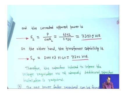
So, therefore, and that corrected apparent power is S 2 is equal to P upon cos theta 2 there for 6942 upon 0.938, so 7397.9 KVA right. So that means, corrected apparent power is 7397.97 KVA therefore, on the other hand the transformer capability is because there are three 2000 KVA transformer, so it actually 2000 into 3 in the power loading capability is 1.2, so it is 7200 KVA right.
