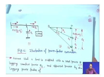
This is your power triangle; this is your power triangle. This Q c you have to make it, this Q c you have to make it, right. So, what will be Q c? Initial power factor was theta 1 right. So, Q is Q c your initial; that means, let me write down here.
