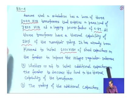
So, next one is an another example right. So, assume that a substation has a bank of three 2000 KVA transformer right, and your the that supplies a peak load of 7800 your what you call KVA right; So, at lagging power factor of 0.89. So, it is a good power factor.
