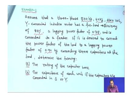
Now, I take another example. Assume that a three-phase 500 horse power h motor operating as 60 hertz and its voltage is 4160 volts that is 4.16 kv right. Star connected induction motor has a full load efficiency of 88 percent 0.88 is efficiency and a lagging power factor 0.75.
