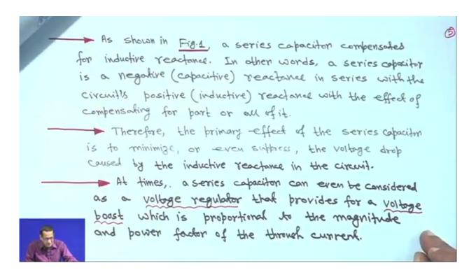
Now, therefore, as shown in figure one I told you that those figure one is series capacitor compensates for inductive reactant because it is x I minus x c right; that is why is compensating in other words a series capacitor is a negative your reactance in series with the circuit with positive react. When negative reactance means it is capacitive positive means it is inductive with the effect of compensating in the part of part or all of it I told you right.
