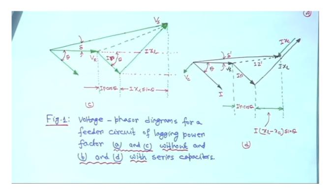
So, if you if you [noise] draw the phasor diagram for this one this is I, this current we are taking as a lagging current for the [vocalized-noise] leading current also we will see, but this is lagging current right. So, corresponding [noise] to this diagram figure a this diagram [noise] this is the phasor diagram we have seen also for approximate voltage drop this thing.
