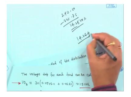
So, in substation voltage was 240.00 and this is 225.75 if you subtract here right so, it will be 14.25 volt right. So, this one we got using this your what you call using that your voltage calculation because it is no iteration here because all currents are known to you and earlier for voltage drop method voltage drop how much you have got 14.264.
