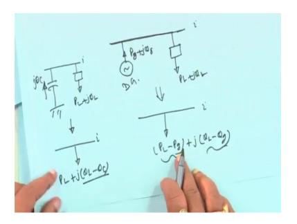
Suppose this is your this is your bus bar right say bus i say this is your load this is your load, this is your P L plus j Q L this is the load right and this is same bus bar suppose generation is connected right. This is P g plus j Q, this is downward this is upward now
