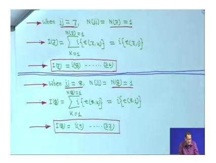
Now similarly when jj is equal to 7, This is the jj is equal to 7 last branch, beyond this branch, I mean there is no other branch in any way. So, this is the receiving node. So, that is a capitalize 7 is equal to small i 8, from that your from this circuit you can easily make out right. So, therefore, jj is equal to 7, Njj is equal to N 7 equal to 1 therefore, I
