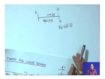
And receiving end node is node 3, and total load fed to this node is p 3 plus a jQ 3 current flowing through this branch is i 2, and impedances is of this branch i 2 plus j x 2 right.
