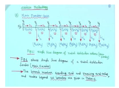
Look at this right; this is the solution methodology; first we will consider the main figure case; that means there is no lateral branches right. So, what will happen that we have taken 8 node problem, if node 1 is a substation, this is your slag bus, this is node 1, this is node 2, node 3, node 4, node 5, node 6, node 7, node 8; the blue ink one right; this is node 8 now.
