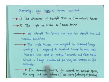
So, generally two types of towers are used. One is the standard your or straight run or intermediate tower, another one the angle or anchor or tension tower. So, the straight run towers are used for straight runs and normal conditions whereas, the angle towers are designed to withstand heavy loading as compared to the standard towers because angle
