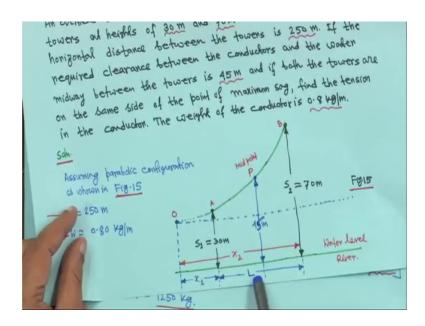
So, that is why assuming parabolic, if it is mentioned catenary or that then you have to do that otherwise if it is not. So, you take L is equal to 250 meter it is given, W - 0.8 kg per meter, that is also given and then h that is difference between these two, this is 30 meter height and this is 70 meter.
