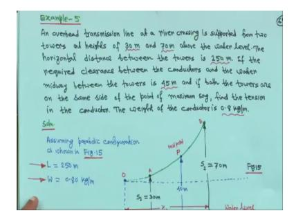
So, next we will take another example. So, here that example -5, here also x 1 will become negative that is why I have made it this way first let me read the problem and over a transmission line at a river crossing is supported from two towers at heights of 30 meter and 70 meter above the water level.
