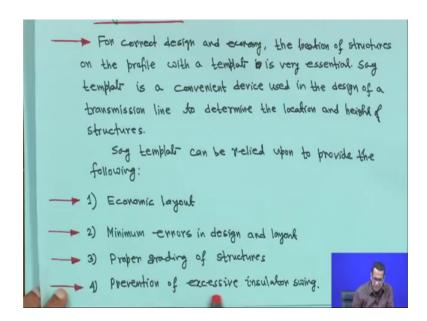
Sag template can be relied upon to provide the following; first thing is economic layout, minimum errors in design and layout proper grading of structures and prevention of excessive insulator swing. All these things will be there on sag template.
