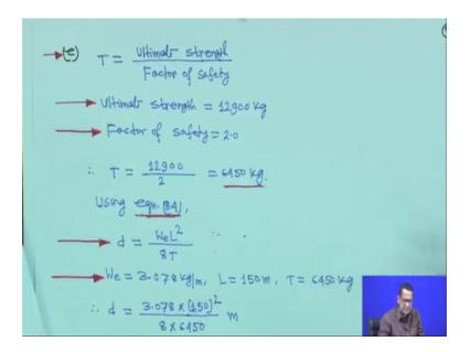
Now, then it factor of safety that term is used. So, factor of safety is given that T is equal to actually ultimate strength divided by factor of safety. Now, ultimate strength is given 12900 kg and factor of safety is equal to 2 therefore, T will be 12900 by 2. So, this you should keep with your mind the T is equal to ultimate strength divided by factor of safety
