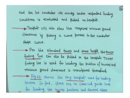
So, for standard towers for normal or average spans the sag and the nature of the curve catenary or parabola, that the line conductor will occupy under expected your loading conditions in evaluated and plotted on template, but the let me tell you one thing for sag template all these things are given it may not be your exactly to your design, but you have some kind of ideas.
