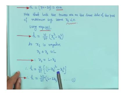
So, h will be 70 minus 30. So, it will be 40 meter h will be 40 meter. Note that both the towers on the same side of the this thing point of minimum sag when x 1 less than equal less than 0, then it is mentioned that both the points are the you know one side of that
