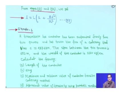
And, in equation – 13, you will get small is equal to capital L in bracket 1 plus 8d square divided by 3L square this is equation 57. So, with these whatever derivation was there for equal supports one is catenary shape, another is parabolic shape these are all the mathematical expression up to equation 57.
