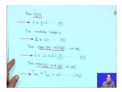
So, from figure -3, again and again not showing the figure -3, it is will we have seen know that C plus d is equal to y therefore, from figure 3 only C is equal to y minus d this is equation 49 therefore, the conductor length that is we know that 1 by 2 is equal S. So, 1 is equal to 2s, s small 2 into small s this is equation 50.
