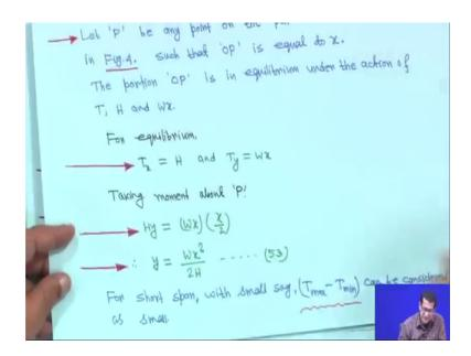
And, if you assume let this is the point P. So, let P be any point on the parabolic curve as shown in figure four. So, P is any point any point such that OP is equal to x. So, this distance this is your OP the distance is your OP is equal to actually this is if you take your S, it will be whatever we are writing that OP is equal to x because of this assumption because we have to just consider the two assumptions.
