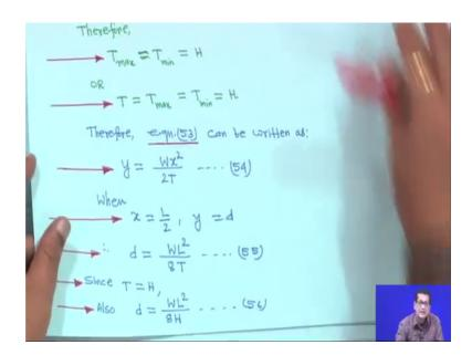
So, t max is equal to T min is H; that means, that we can write that one also T. So, T is equal to T max is equal to T min is equal to H therefore, equation 53; that means, this equation y is equal to Wx square by 2H, we can write this equation that as T is equal to ultimately it is coming T is equal to H therefore, we can write y is equal to Wx square upon 2H this is equation 53. So, we can write this equation y is equal to Wx square upon 2T is because H is equal to T this is equation 54.
