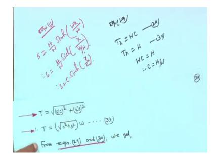
Equation 29, so, 29 actually T x is equal to W into C and 30 actually T x is equal to H this is equation 29 and this is 30; that means, WC is equal to H; that means, C is equal to H by W, that is why you are writing this in this equation that in this equation that C is equal to H by W.
