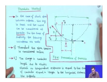
Now, suppose if it is a parabola now whatever we have seen that is basically general case now if it is a parabola. So, equal y your shapes are this is the same level distance is L and this is the maximum sag d some point P we have taken. So, tension T y acting along this direction upward and here it is your T x is the horizontal tension angle between this is the tension T tangential it is working.
