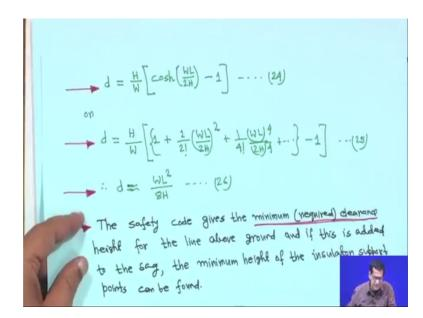
Then what you will get this equation that that if you substitute here then you will get, d is equal to because y is equal to d d is equal to H upon W cos hyperbolic W l upon 2 H because x is equal to l by 2 minus 1 this is equation 24.
