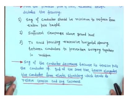
But at the same time tension elongates the conductor from elastic stretching, which tends to relieve tension and sag increases right.
