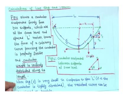
Now, these are some simple thing, now calculation of line sag and tension, actually we have taken a catenary shape these are symmetrical although my handwriting is slightly this way, but this side and this side it is symmetrical right. So, this is your suppose it is your both the side this is tower side this one and this one, they are of equal height right. So, this is the first thing.
