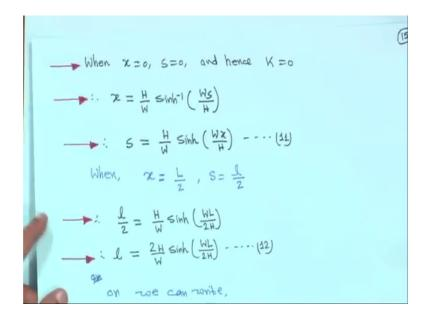
Though in this case your S k will become 0 so, therefore, x is equal to H upon W sin H inverse that is sin hyperbolic inverse Ws by H or S is equal to we can write H by W sin hyperbolic Ws by H, I mean cross multiply Ws by H and then you just you simplify. So, we are writing S is equal to this is equal to H by W sin hyperbolic Ws by H this is equation 11 right.
