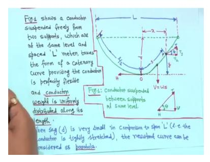
And conductor weight is uniformly distributed along it is line, actually total length of the conductor is small l. So, from here to here we have this is l by 2 this side also total is l by 2 right, but we have taken some point your p. So, in this case that when sag your d is very small when d is very small in computation to span l, that is that conductor is tightly stretched, the resultant curve can be considered as a parabola right.
