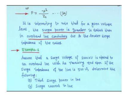
So, now it is interesting to note that for a given voltage level, the surge power is greater in cables than in overhead line conductors due to the smaller surge impedance of the cable, in the cable the surge impedance is small right. So, that is why the given voltage level the surge power is greater in cables because, your denominator is less right than in overhead line conductors and due to the smaller surge impedance of the cable right, slowly we will go into the deep of it.
