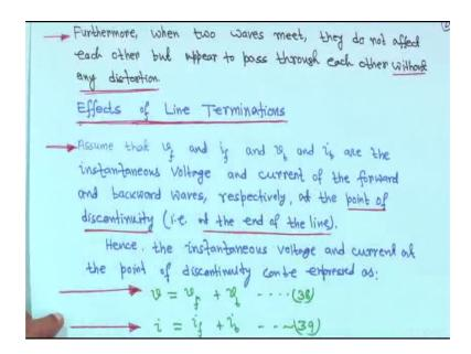
If they both the waves meet they do not affect each other, but appear to pass through each other without any distortion, I mean when both are moving I mean one is if 1 is moving this way another wave is moving this way there will be no distortion actually, without any distortion they pass you what you call through each other without any distortion this is very interesting right.
