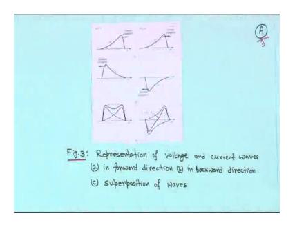
So, this here this one is the forward propagation this figure. So, I have taken from book right. So, because then see figures are symmetrical it will be easy for you to understand. So, this is a forward propagation this is voltage here this is x is increasing for this side right and this is forward propagation this is i f the current right shape banged by your dimension different, but shape is remaining same values may be different shape is remain same.
