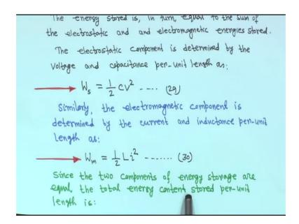
So; that means, the electrostatic component is determined by the voltage and capacitance per unit length is you know that it is w s is equal to half c v square this is equation 29 this is electrostatic one and for electromagnetic component is it can be determined by the current and inductance per unit length we know that w is equal to half Li square.
