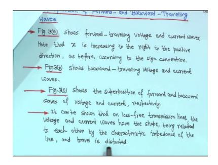
So, now the super position and figure 3 is shows forward travelling voltage and current wave this is your figure a b and figure c right. So, in this case the travelling wave current note that x is increasing to the right in the positive direction I told you this way x is increasing right and as before according to the sign convention; figure 3 b shows backward travelling voltage and current wave this is backward your propagation voltage wave and this is current wave right.
