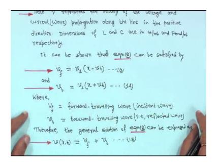
Now here gamma actually represent the velocity of the voltage and current wave, that is propagation velocity of voltage and current propagation along the line this is the gamma right; in the positive direction. Dimension of L and C same as the Henry per meter and
