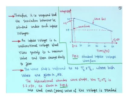
So, lightning is a lightning stroke particularly is a very strong phenomena where in you have to put it the power system. So, I will come to this figure later on therefore, it is required that the insulation behaviour we studied under such impulse voltages; that means, that is your what you call that whenever they go for; suppose manufacturers when the manufacture transformers for example, say they go for level phase stage that your impulse stage because it will last for micro second.
