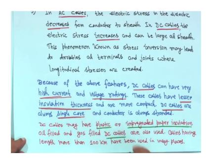
Now, so in AC cables the electric stress in the electric; in the dialectic decreases from conductor to sheath; that we have near the surface of the conductor that electric stress is
