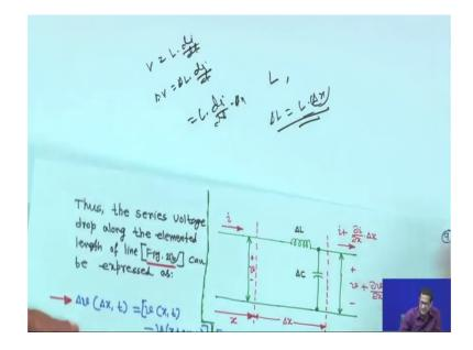
So, inductance is L and length is say d x delta x rather delta x; then delta L actually is equal to L into delta x. So, this is your delta L; that means, this L we are representing say Henry per meter say; may be Henry or Henry whatsoever. So, this is actually delta L same is applicable for capacitor.
