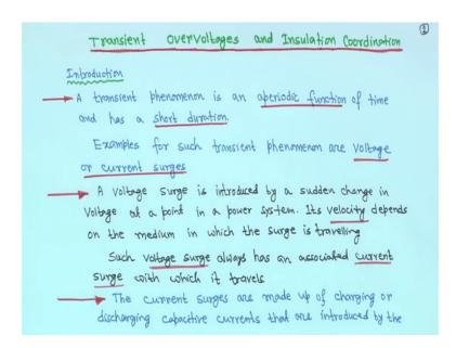
So, this is a new topic that transient over voltages and insulation coordination; let us see first what exactly it is. So, a transient phenomena is an aperiodic; function of time and has a short duration you know that.
