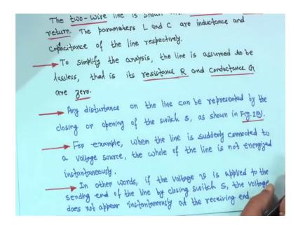
Shown with one phase and neutral return in one phase and neutral return; the parameters L and C you know inductance and capacitance of the line respectively. So, to simplify the analysis what we have done resistance and conductance G; we have assumed zero that is they are neglected you just for the purpose of you know explanation. So, any disturbance on the line can be represented by the closing or opening of the switches as shown in figure 2 a.
