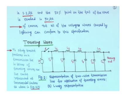
I told you this one of course, not all of the voltages waves caused by lightning can conform to this specification. Even if you go for laboratory test for impulse voltage test; you will not find that your what you call 1.2 or 50; it may change, but this is standard one of the travelling wave.
