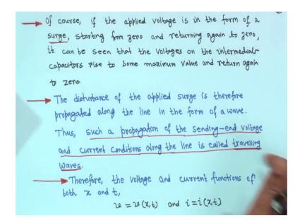
So, done and if the applied voltage is in the form of a surge suppose if the applied voltage is in the form of a surge; say this starting from 0 and returning again to 0. Suppose it is just a your what you call it is form of a surge starting from 0 and returning again to 0. Therefore, it can be seen that the voltages on the intermediate capacitor rise to some maximum value and again return to 0.
