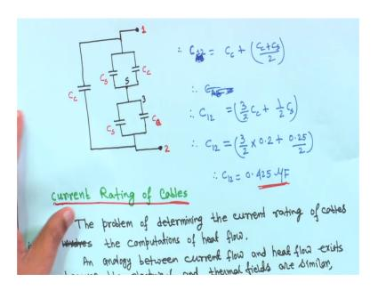
So, this is 1 and 2 right between 1 and 2 C c it is there and s and 3 is a common point, where just to show it differently that is why s and 3 is a separate where is a common point.
