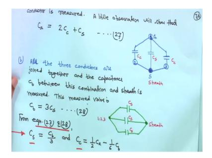
So, what it is telling that any 2 conductors are connected to the sheath, suppose any 2 conductor; what you call there are 1 2 3; three conductors are there. So, any 2 conductor this is sheath, it is taking as a your what you call this is actually it is a sheath it is a common point right because, it is a common if this 1 nothing is there in between that it is a common point.
