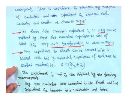
So, consequently there is a capacitance C c that I showed you that this capacitance is C c right, between any 2 pairs of conductor and capacitance C s between each conductor and
