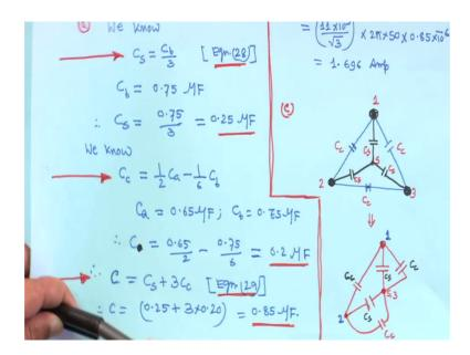
Now, this we know that C s is equal to Cb by 3 do not see this 1, no need to see this 1 you look at that C s is equal to Cb by 3 from equation 28, Cb is given 0.75 microfarad therefore, C s will be Cb by 3. So, 0.7 by 3 0.75 by 3 that is your 0.25 microfarad and we know also C or C c is equal to half Ca minus 1, I mean this equation is actually your C c is equal not this 1, C c is equal to half C minus 1 upon 6 Cb this equation you have derive.
