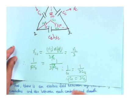
Suppose this is your capacitor this is delta connection right and this is your, this point is 1 and this is 2 and this point is your 3 right, this is 3 conductor their capacitance is this is C c and this is your C c right, so if I convert to star right.
