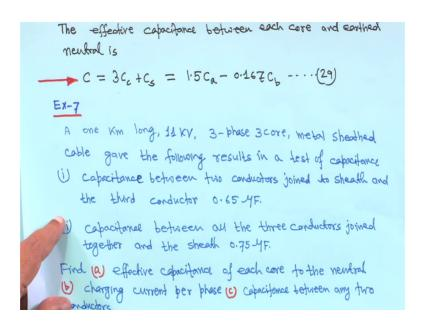
Therefore, that effective capacitance, the effective capacitance between each core and earthed neutral is C is equal to 3 C c plus C s this we have seen.
